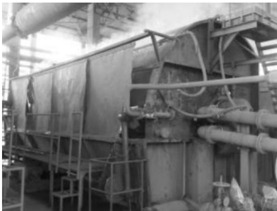
Figure 1. Red Mud Vacuum Filter at Alunorte
