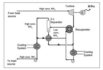
Figure 2. Simplified schematic for the Kalina cycle for low temperature applications.
