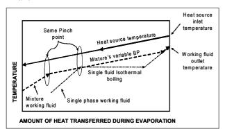
Figure 1. Temperature profiles during heat transfer in the evaporation step of the cycle.
