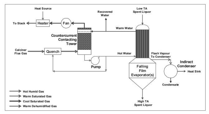
Figure 4. A flowsheet for the recovery of waste heat and water from calciner flue gas.
