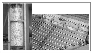
Figure 5. (a) Pilot scale Turboscrubber and (b) impingement tray for tray tower (Lisbon Engineering, with permission).
