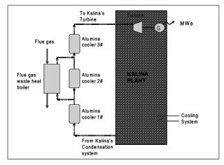
Figure 3. Heat recovery configurations studies at Alcoa's Jamalco Refinery
