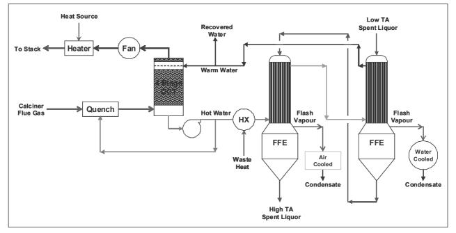
Figure 6. Calciner waste heat recovery with air cooled condensers for greater water recovery.
