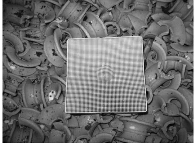
Sample of CR20 placed in RTO for testing
