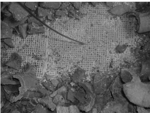
Damaged top layer of ceramics after 4 months operation
