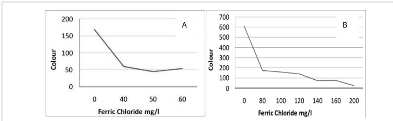
Figure 4 Removal Performed by Veolia using Actiflo Process Simulation using Micosand, Ferric Chloride and Flocculant on A) Clarifier Overflow and B) Decant Pond Overflow
