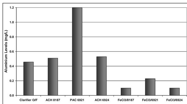
**Figure 6 ICP Analyses for Aluminium – Impact of ACH and PAC on Clarifier Overflow**
