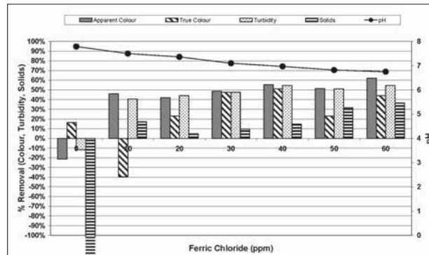
Figure 9. % Removal of Colour, Turbidity and Solids: Impact of Ferric Chloride with Nalco Optimer 83372 (1ppm)
