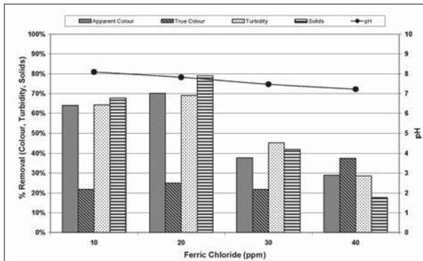
Figure 8 % Removal of Colour, Turbidity and Solids: Varying FeCl3 with Nalco Optimer 83372 (1ppm)
