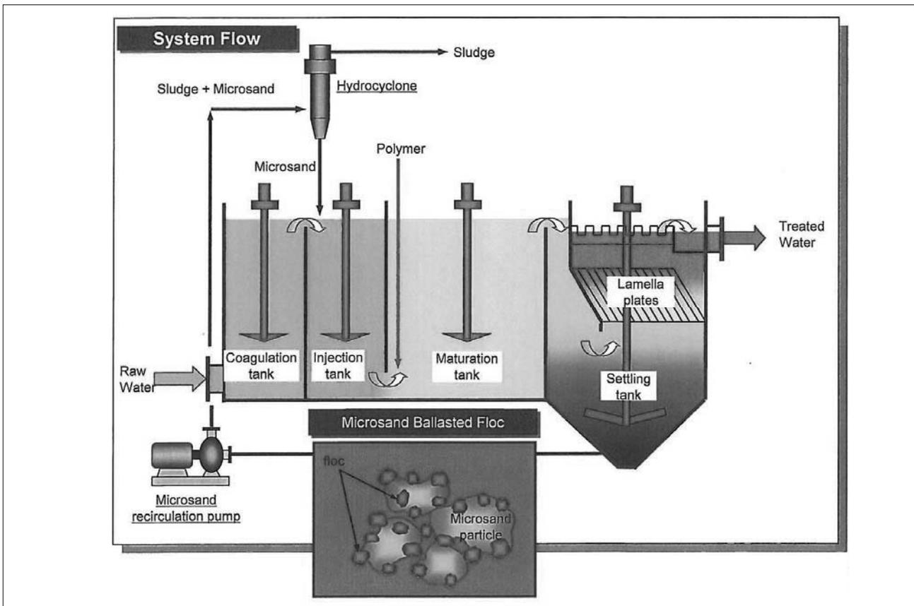
Figure 3 Diagrammatic System Flow of Veolia Actiflo
