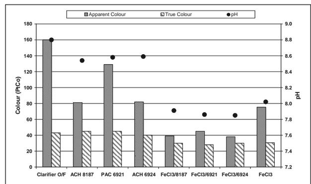
Figure 5 Clarifier Overflow: 20 ppm PAC/ACH and 30 ppm Ferric Chloride and 1 ppm Nalco 833722
