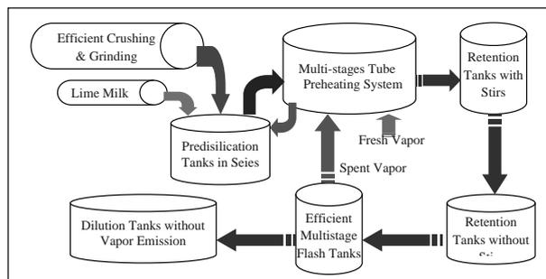
Fig.8. The best energy saving intensifying digestion process scheme
