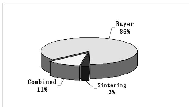
Fig.2. Production proportions of various processes in China
