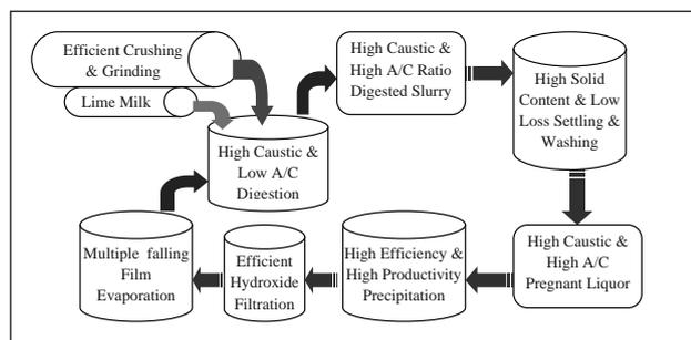
Fig.7. High cycling efficiency Bayer process scheme
