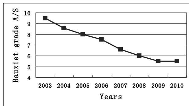
Fig.6. Bauxite grade reduction for the northern refineries in China
