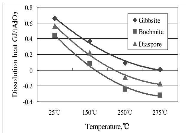
Fig. 3. Dissolution heat for different alumina minerals in caustic solution
