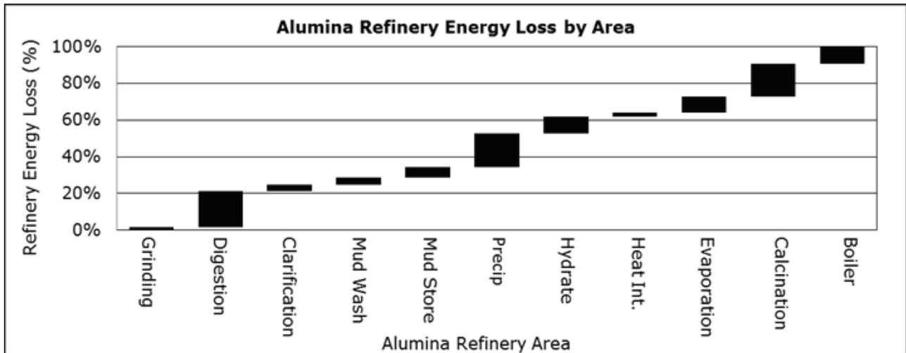
Using this approach, it is possible to narrow down both the key focus Bayer Process Areas for the recovery or minimisation of energy losses, as well as the pathway by which energy is lost, which then forms the basis for energy improvements in further flow sheet developments.
