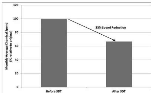
Figure 3. Chemical savings achieved through the implementation of 3D-Trasar technology on a single cooling tower from refinery A above. Average monthly spend relative for the 9 months after 3D-Trasar installation plotted relative to average spend for 12 months prior.
