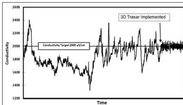
Figure 1. Variation in conductivity over time (3 months data is shown) as measured in an operating cooling tower. Implementation of 3D-Trasar technology results in much tighter process control.
