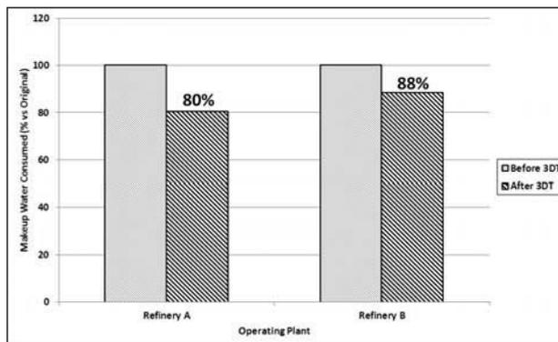
Figure 2. Water savings from implementation of 3D-Trasar technology on a series of cooling towers at two separate refineries. Amount of makeup water required before and after implementation of 3D-Trasar technology is plotted relative to the original amount of makeup water used.
