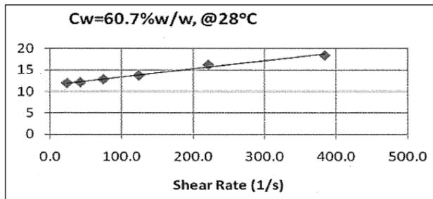
Figure 2: Rheograms of a Vietnam bauxite slurry
