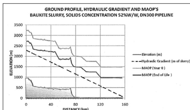
Figure 4: Pipe profile, Hydraulic gradient and MAOP's.
