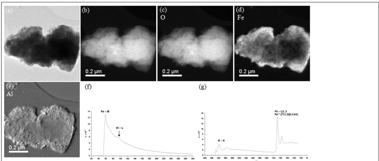
**Figure 10.** (a) Energy filtered electron micrograph of part of a maghemite particle, (b) thickness map, (c) oxygen map, (d) iron map, (e) aluminium map, (f) EELS for iron and aluminium, (g) EELS for oxygen and iron (ferric  $\text{Fe}^{3+}$ ).
