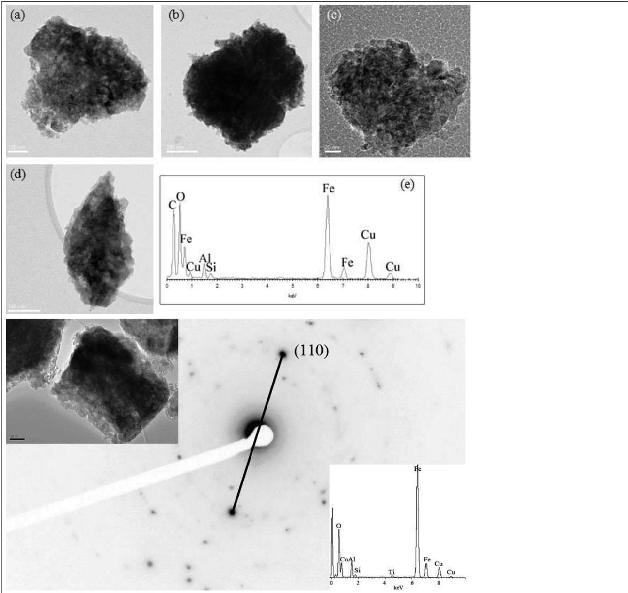
**Figure 9.** Electron micrographs of hematite particles (a, b, c, d) showing that particles are complex aggregates of ~20 nm platey subcrystals (e) EDS spectrum of the particle shown in (b) indicating substantial Al substitution for Fe. The Si and Cu peaks are due to the supporting film and grid respectively. The crystal of Al-rich hematite shown at the bottom of the figure is resting on its (001) face as indicated by the electron diffraction pattern.
