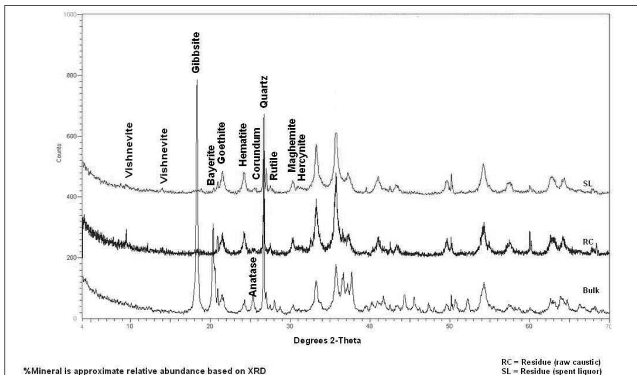
Figure 2. XRD patterns of UWA01-10 bauxite bulk sample and residues, with inset tables showing calculated %minerals and %Al in minerals. Please note that the XRD technique does not give highly accurate or precise measures of abundance or composition so the data in the table are approximate.
