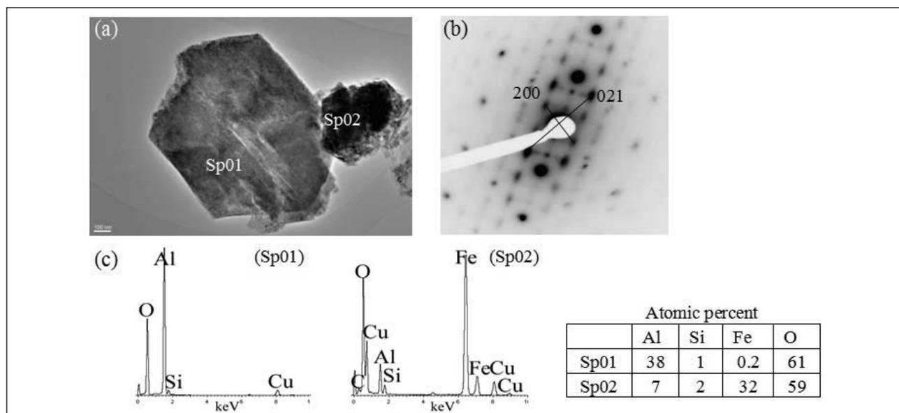
Figure 3. (a) Electron micrograph of gibbsite (Sp01) and aluminous goethite (Sp02) particles, (b) electron diffraction pattern of the gibbsite particle (Sp01) and (c) x-ray spectra of the gibbsite particle (Sp01) and the aluminous goethite particle (Sp02) (The Si and Cu peaks are due to supporting film and grid respectively).
