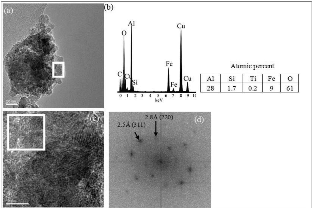
Figure 6. (a) Electron micrograph of a hercynite particle, (b) x-ray spectrum of the particle (The Si and Cu peaks are due to the supporting film and grid respectively), (c) high resolution electron micrograph of the indicated area of the particle showing a lattice image and (d) Fourier transform diffraction pattern for the indicated area in (c).
