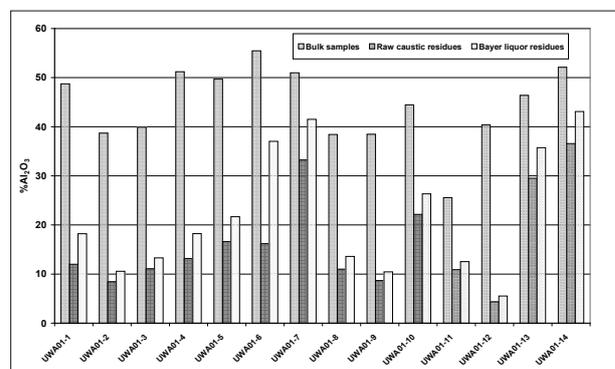
Figure 1. %Al<sub>2</sub>O<sub>3</sub> in bulk samples and caustic digest residues, determined by XRF.
