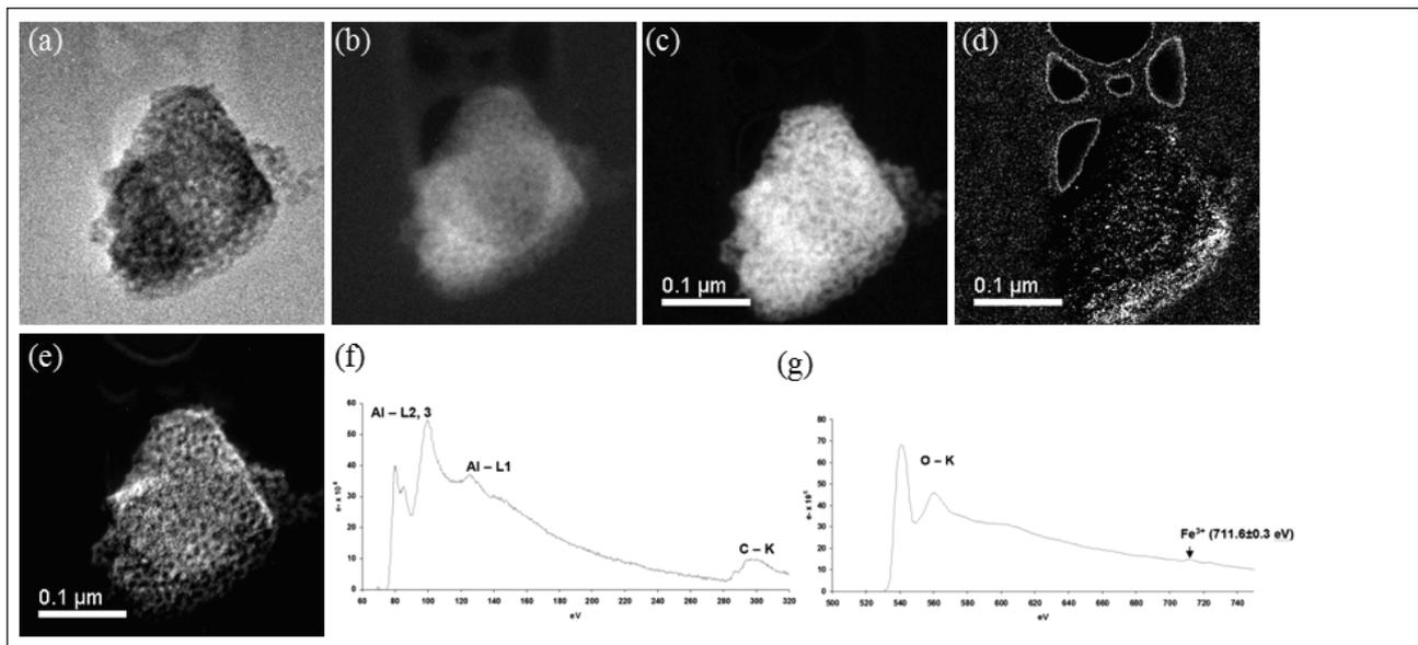
Figure 5. (a) Energy filtered electron micrograph of a corundum particle, (b) thickness map, (c) oxygen map, (d) iron map, (e) aluminium map, (f) EELS for aluminium and carbon, (g) EELS for oxygen and ferric iron.
