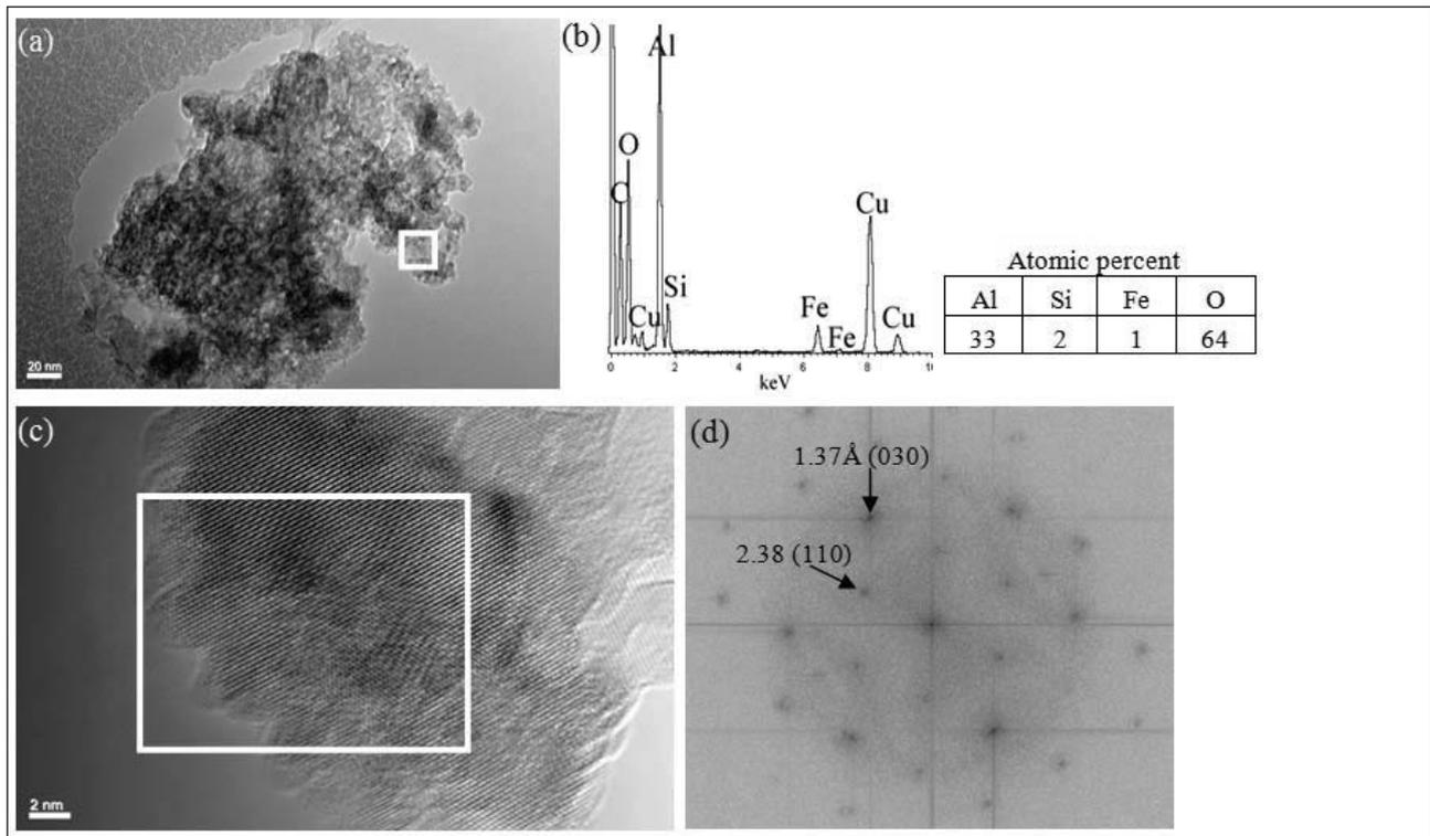
Figure 4. (a) Electron micrograph of a corundum particle, (b) x-ray spectrum of the particle indicating minor substitution of Fe for Al (The Si and Cu peaks are due to the supporting film and grid respectively), (c) high resolution electron micrograph of the area indicated by the white square in (a) and (d) Fourier transform diffraction pattern of a region of the corundum particle indicated by the white square in (c).
