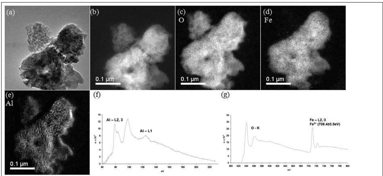
Figure 7. (a) Energy filtered electron micrographs of the hercynite particles, (b) thickness map, (c) oxygen map, (d) iron map, (e) aluminium map, (f) EELS for aluminium and (g) EELS for oxygen and iron which corresponds to ferrous (Fe<sup>2+</sup>).
