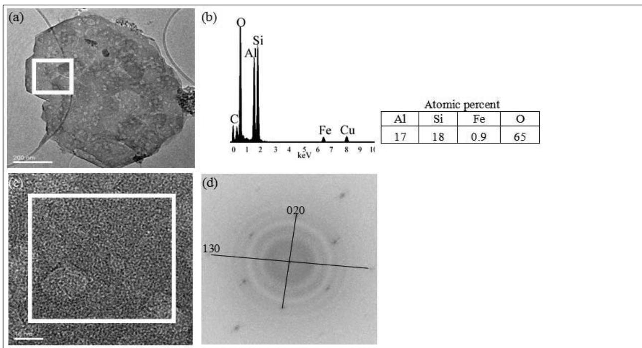
Figure 12. (a) Electron micrograph of a kaolin particle, (b) x-ray spectrum of the particle (The Cu peaks are due to the supporting grid), (c) high resolution electron micrograph of the area within the white square in (a) and (d) Fourier transform diffraction pattern of the region of the kaolin particle indicated by a white square area in (c).
