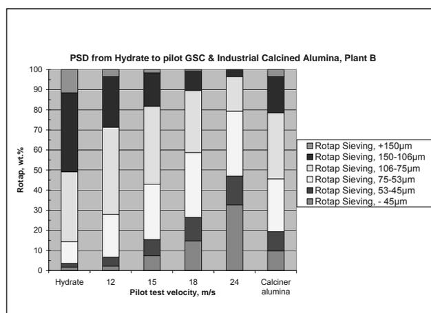
Figure 5a. Hydrate and Alumina from Plant B.
