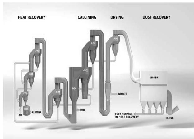
Figure 1a: FLS Gas Suspension Calciner (GSC) flow sheet.
