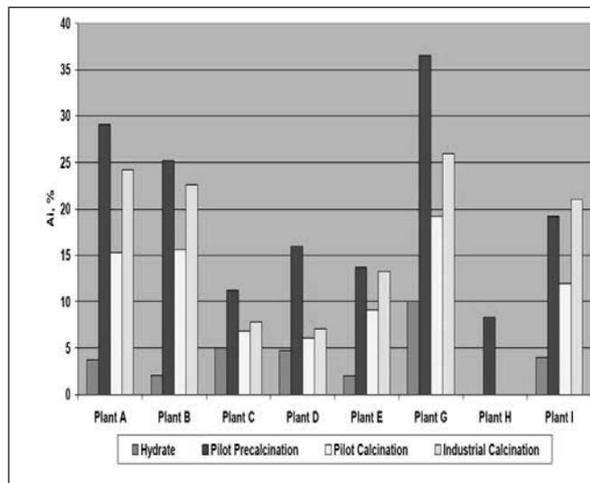
Figure 4a: Attrition Index versus Degree of Calcination.
