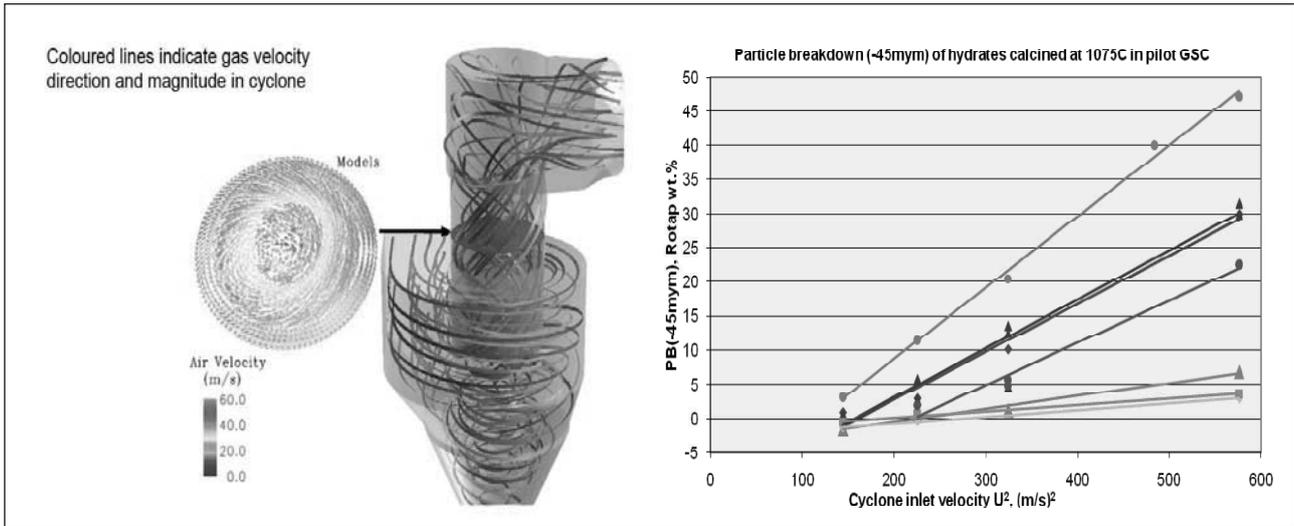
Figure 6a. CFD Model of Cyclone
