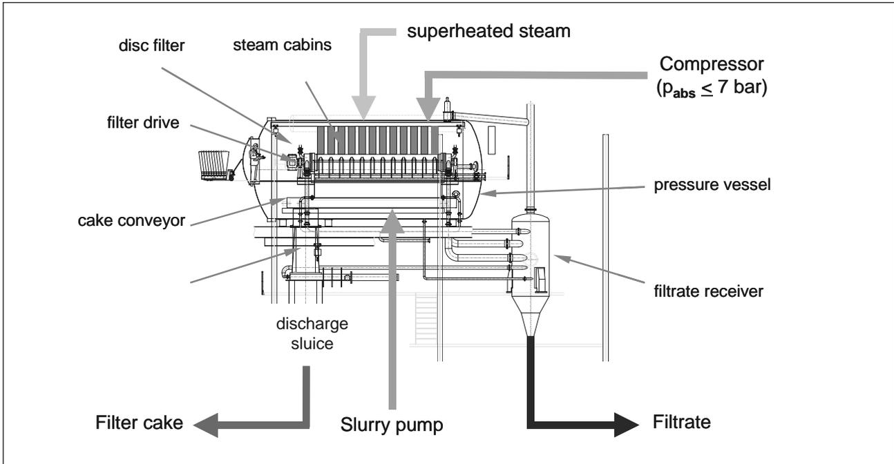
Figure 1: Schematic view of Continuous Pressure Disc Filter with steam cabins for steam pressure filtration
