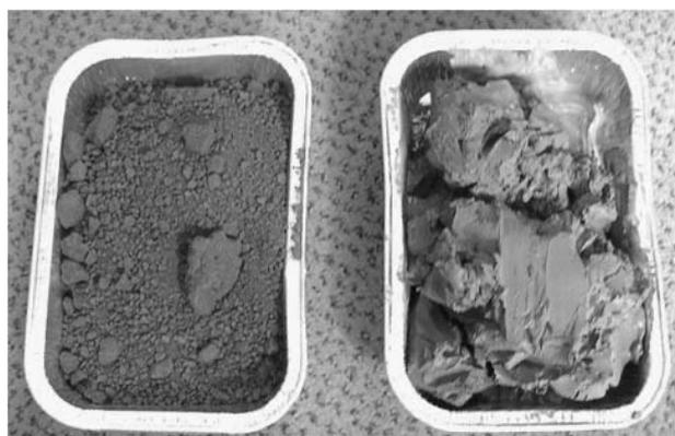
Figure 4: Filter cakes of red mud: pasty and sticky with a moisture content of 35 wt-% (vacuum filter) and sandy material with mc = 23 wt-% from Hi-Bar Steam Pressure Filtration
