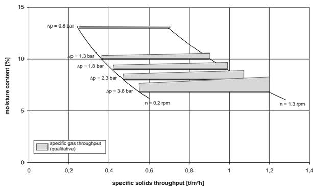
Figure 2: Residual moisture content versus specific solids throughput for different values of pressure difference  $\Delta p$  and filter speed  $n$  (zinc ore)
