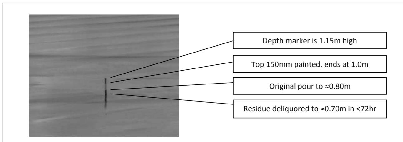
Figure 3. Example of residue deliquoring in an area 48-72 hours after pouring at 56 wt% solids. Deliquoring rate calculated to be 14-21 m<sup>3</sup>/Ha/hr, or an increasing solids content of 1.7-2.5 wt%/dy.
