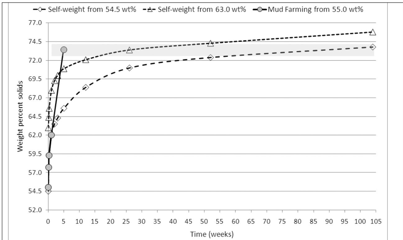
Figure 5. Effect of an enhanced AST consolidation regime on residue consolidation rate versus natural consolidation rates. Shaded area between 72.5 and 74.0 wt% solids indicates target solids content for continued construction.
