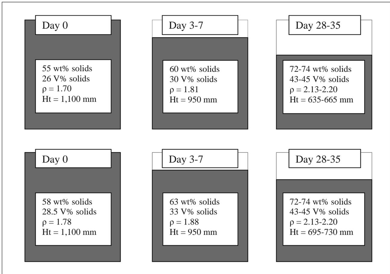
Figure 4. Progression of consolidation with discharge at 55 or 58 wt% solids.
