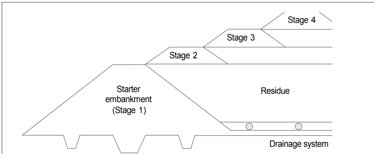
Figure 1. Schematic of upstream embankment construction method
