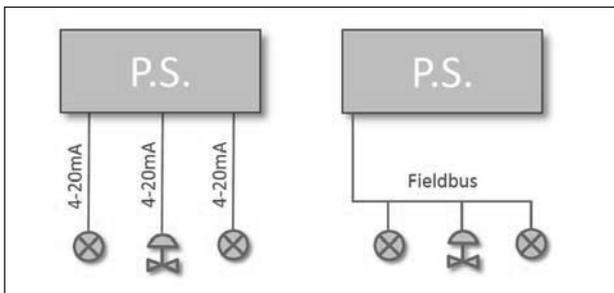
Figure 1: 4-20mA vs. Fieldbus
