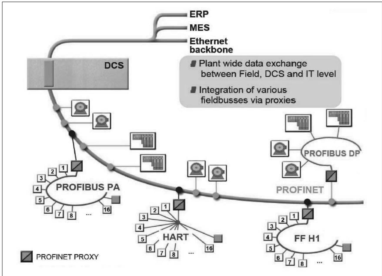
Figure 5: Profinet technology integration
