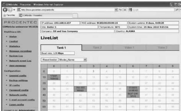
Figure 7: Web Browser Screen for Profibus Network Monitoring
