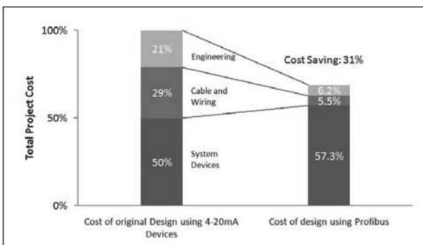
Figure 2: Cost Comparison between conventional installation and Profibus
