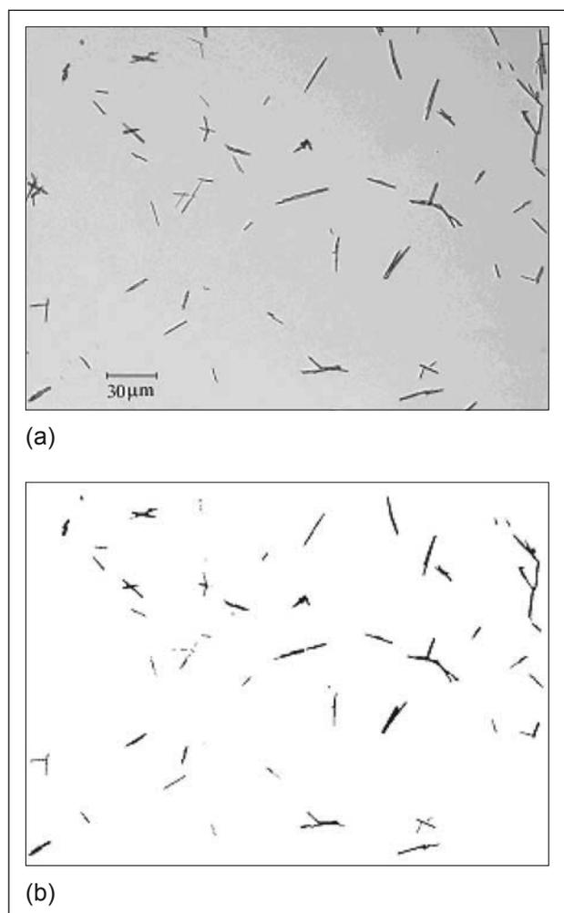
Fig. 1. Optical microscopy image (5 Mpix resolution) of needle-like oxalate crystals: (a) original digital image, and (b) binary image with the highlighted objects identified by the developed image analysis algorithm.
