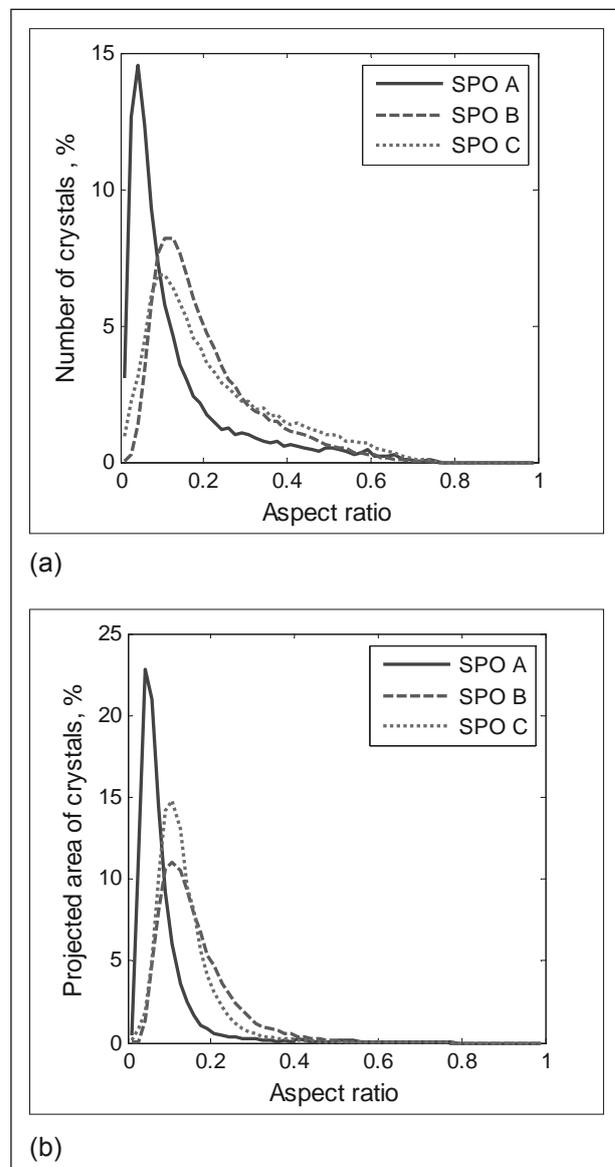
Fig. 6: Number-based aspect ratio distributions (a), and projected area-based aspect ratio distributions (b) for three different types of oxalate crystals.
