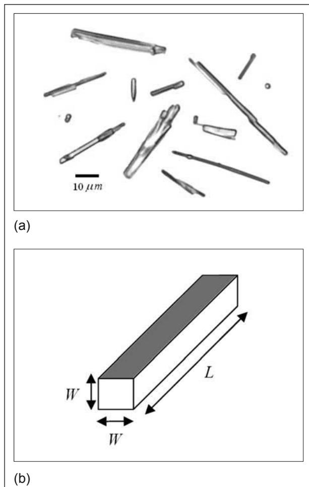
Fig. 2. An optical microscopy digital image, 40x magnification, of needle-like oxalate crystals (a), and a two-dimensional rectangular approximation of a 3-D crystal (b).
