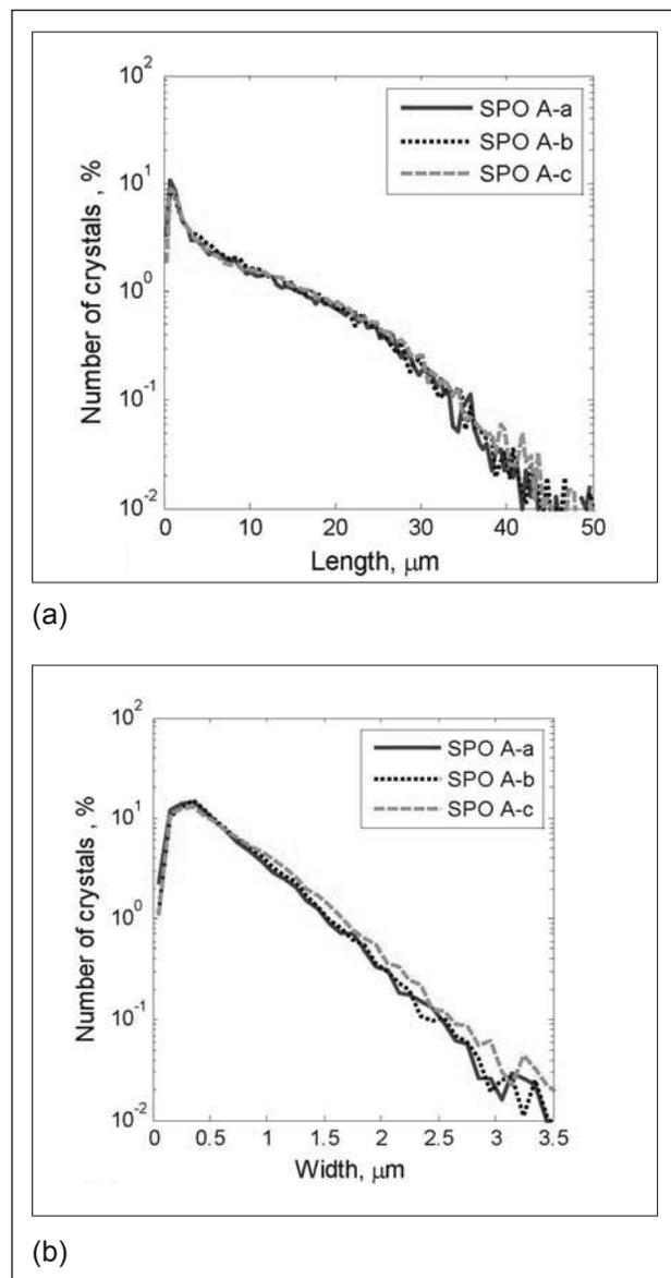
Fig. 4: Reproducibility of measured length (a) and width (b) distributions of ‘SPO A’ oxalate crystals.
