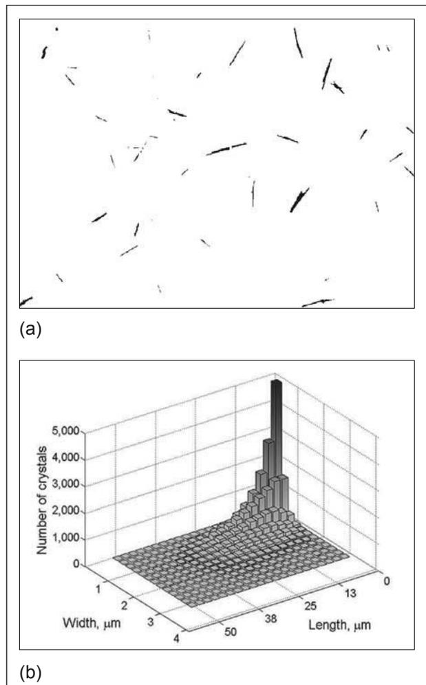
Fig. 3. Needle-like crystals identified after applying a non-dimensional rectangularity filter (a), and a complete 2-D size distribution of identified needle-like oxalate crystals (b).
