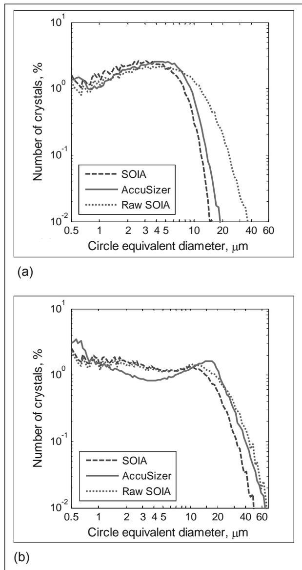
Fig. 9: AccuSizer and SOIA number-based crystal size distributions for: (a) 'SPO B' crystals, and (b) 'SPO C' crystals.
