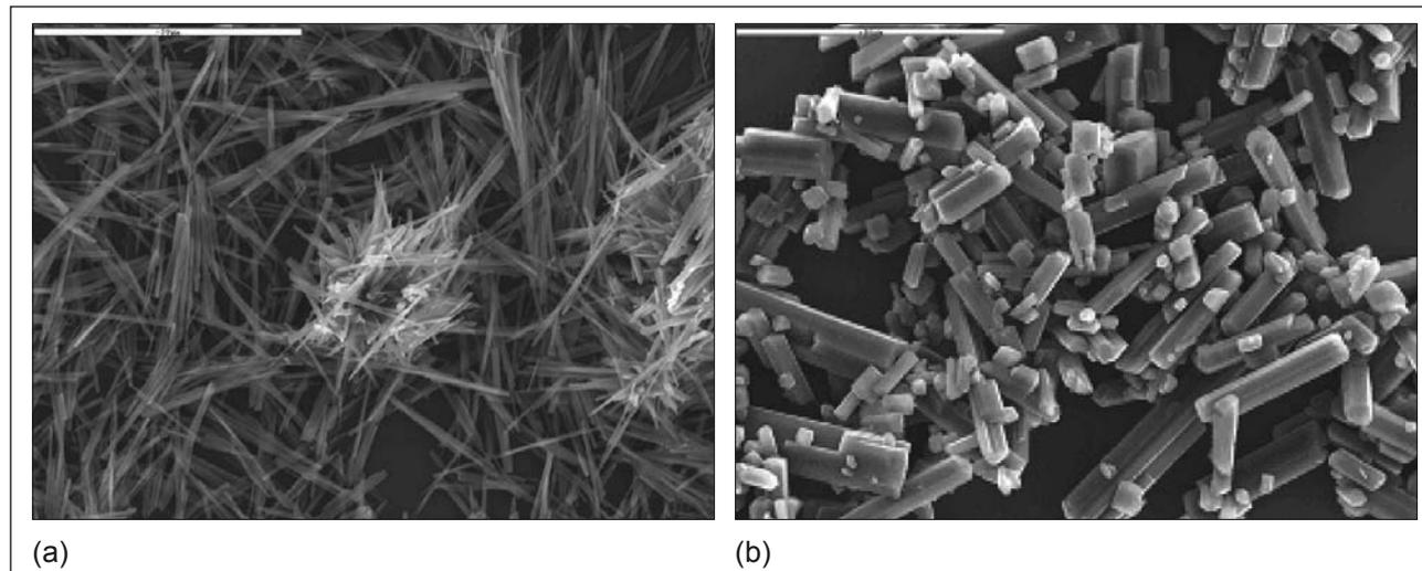
Fig. 7. SEM images of laboratory prepared oxalate crystals: (a) 'SPO A'; and (b) 'SPO C'.
