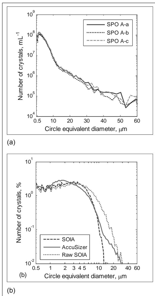
Fig. 8. Repeated AccuSizer measured number-based 'SPO A' crystal size distributions (a), and AccuSizer and SOIA number-based 'SPO A' crystal size distributions (b).
