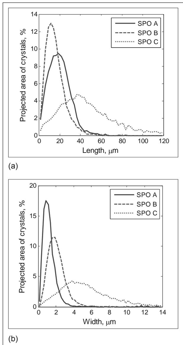
Fig. 5: Projected area-based length (a) and width (b) crystal distributions for three different types of oxalate crystals.
