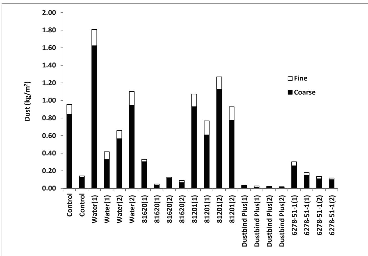
Figure 1: Dust (kg/m²) formed below the surface crust of surface-treated red mud samples. The number in brackets denotes the weekly application frequency.
