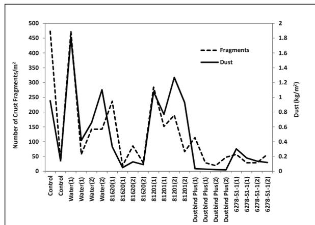
Figure 2: Relationship between surface crust cracking and dust formed.
