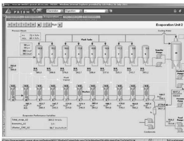
Figure 2. Overview model-based process screen
