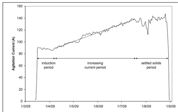
Figure 4 Agitation current for a post-interstage Swirl Flow agitator
