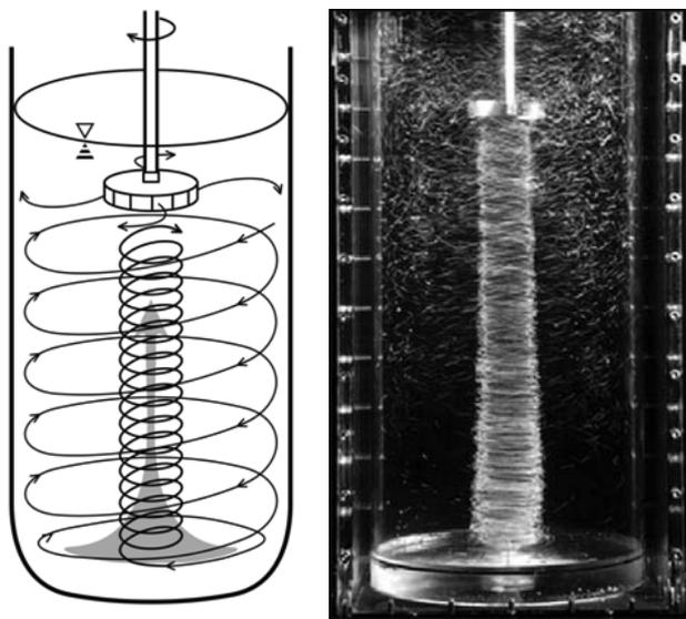
Figure 1 (a) Diagram of flow patterns (b) Flow visualisation of Swirl Flow (Courtesy of CSIRO)
