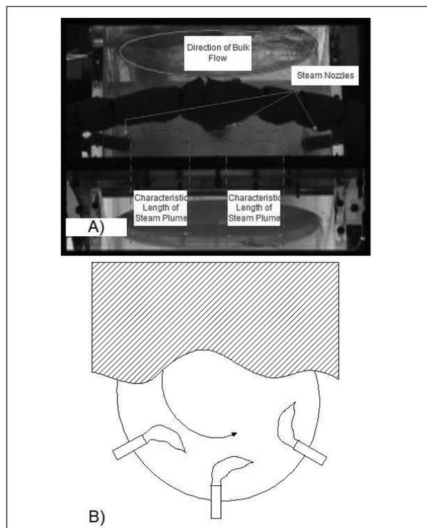
Figure 8: Close up and schematic depiction of steam nozzles showing A) length of steam plume and B) the skewed nature of the steam jets
