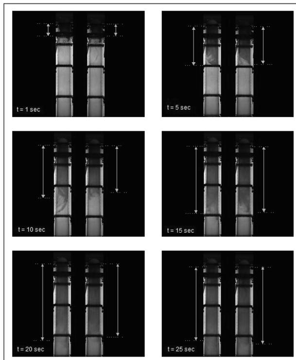
Figure 4: Dye tracing tests of the digester at selected time intervals. The left hand digester in each frame is the 52 mm nozzle case; the right hand side is the 40 mm case.
