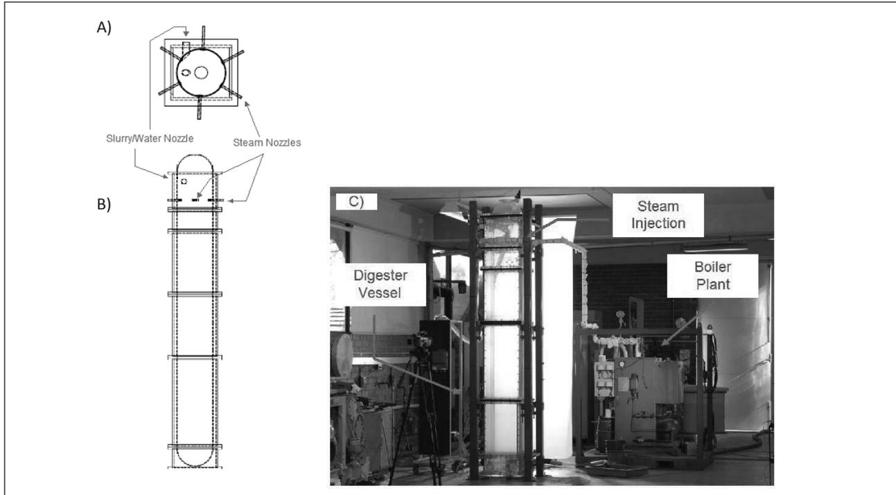
Figure 1: Schematic Diagram of the Digester, top view A), Side View B) and Photograph of digester Perspex model and steam boiler plant C).
