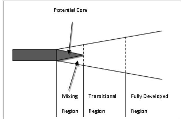
Figure 7: Flow regions of a turbulent free jet.
