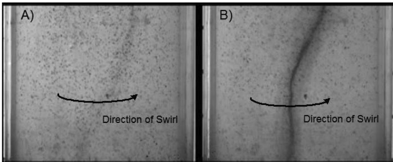
Figure 2: Flow visualization of mid section of digester, fluid laced with polystyrene beads A) 52 mm nozzle and B) the 40 mm nozzle.
