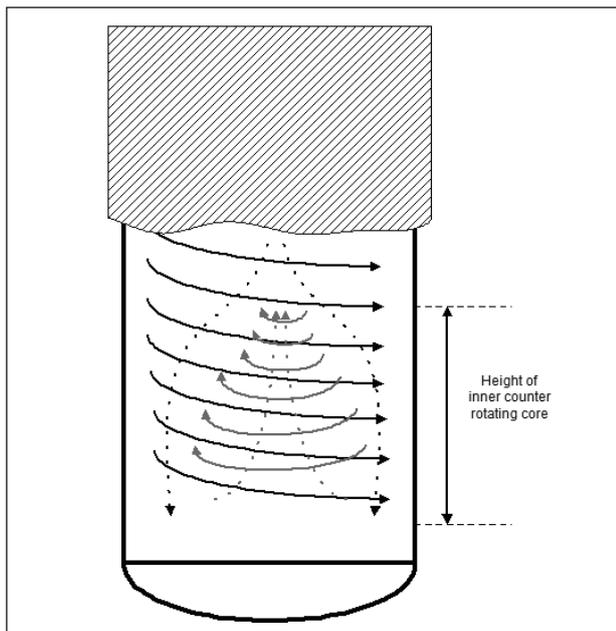
Figure 3: Schematic diagram of inner rotating counter vortex.
