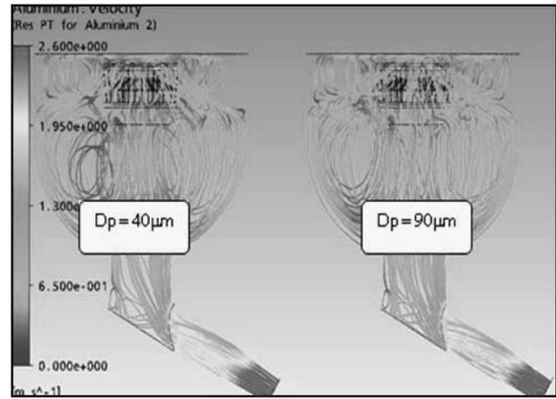
Figure 8 – New Design CFD Analysis - Velocity at Outlet
