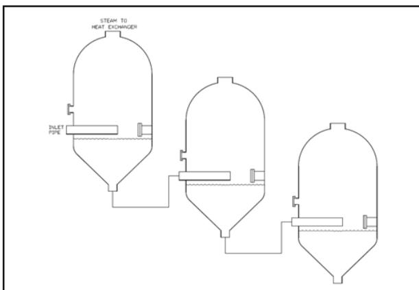
Figure 3 - Side Entry - staged vessels
