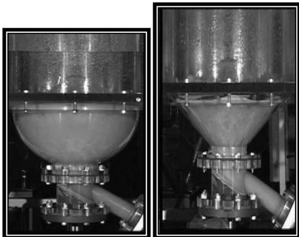
Final test runs incorporated isolating the circulating flow for a period of several minutes to allow particle settlement through the test rig and external piping and reinstating the pump flow, to gauge the ability of the system to remobilise the solids particles.
