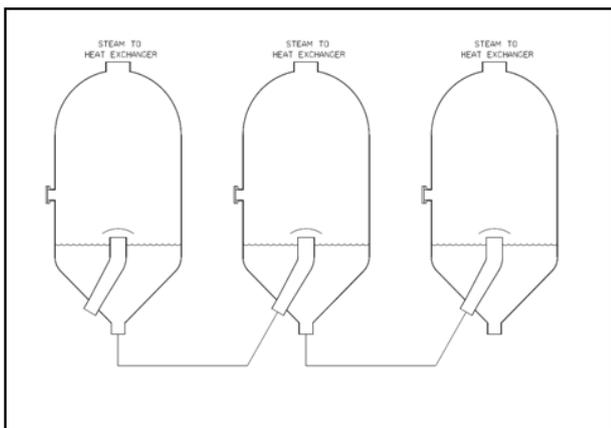
Figure 5 – Bottom Entry – Multiple Vessels
