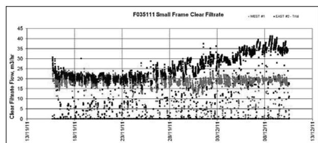
Graph showing the flow data from the Nov. Trial. The standard frame was the West #1 data, the sine shape frame was the East #2 data
