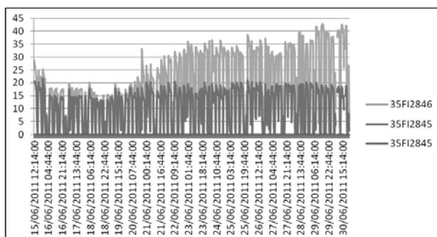
Flow graph showing the flow from each filter cycle, 35F12846 is the sine shape frame and 35F12845 is the standard frame.
