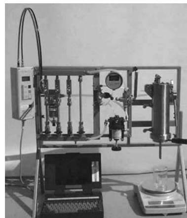
Figure 2: The laboratory pressure filter cell FILTRATEST
