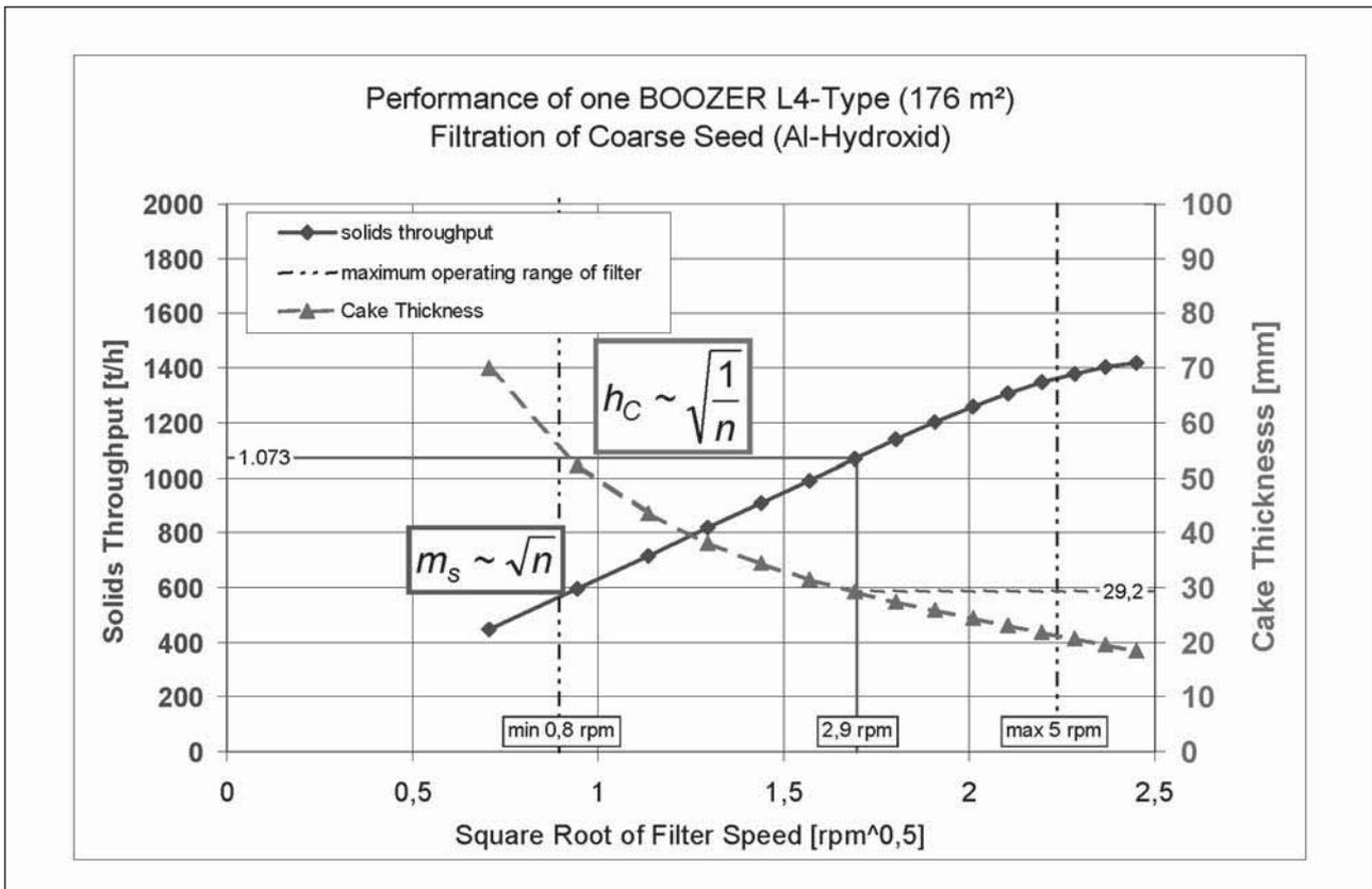
Figure 5: Solids throughput of a Boozer disc filter versus square root of filter speed  $n$  and cake height  $h_c$  (Al-hydrate coarse seed filtration)
