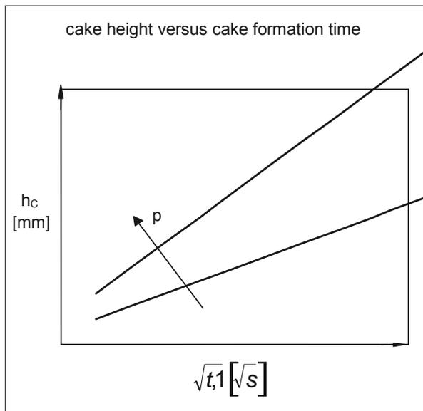
Figure 3: Interrelationship between cake height  $h_C$  and filtration time  $t_1$  in case of incompressibility
