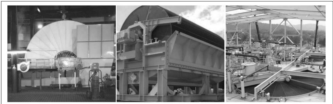
Figure 1: BOKELA rotary filters: Boozer vacuum disc filter (left), drum filter (mid) and pan filter (right)
