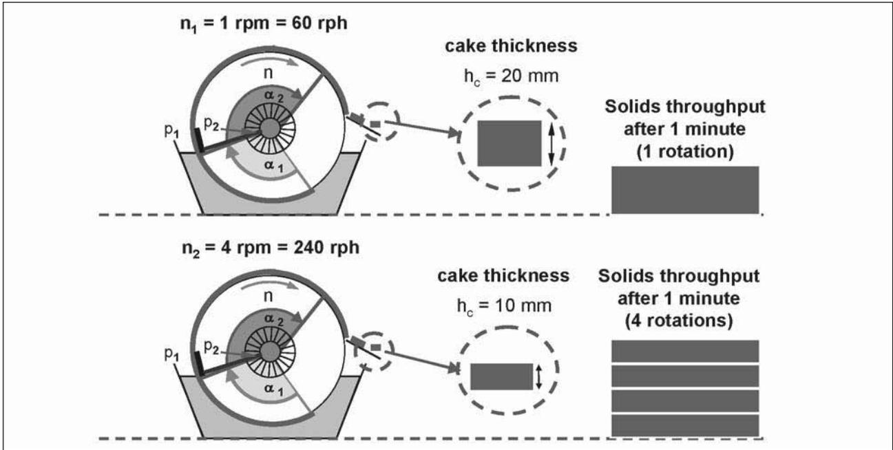
Figure 4: Filter speed is the throttle of filtration
