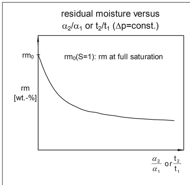
Figure 7 and 8: Residual moisture displayed as throughput function and as function of the interrelation between dewatering- and cake forming time
