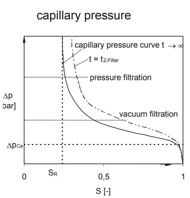
Figure 6: Capillary pressure curve
