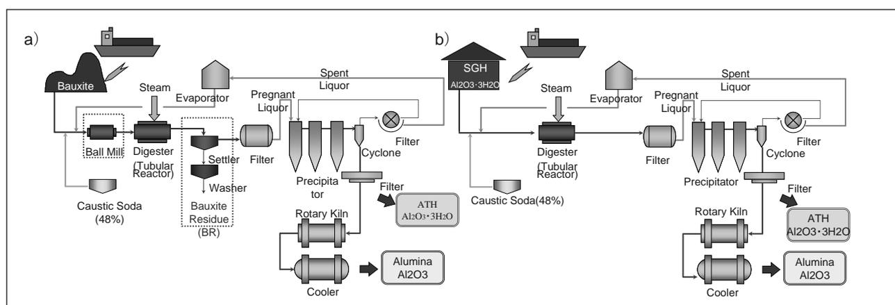
Figure 1 shows Bayer process in Ehime plant before/after feedstock conversion.
