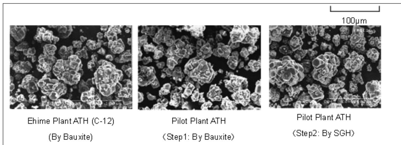
Figure3. SEM images of Ehime plant and pilot plant ATH
