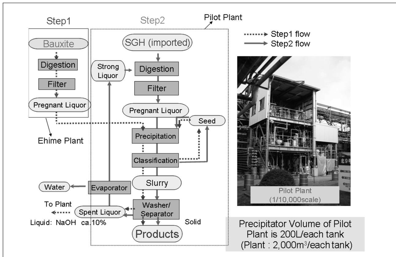
Figure2. Experimental procedure in pilot plant
