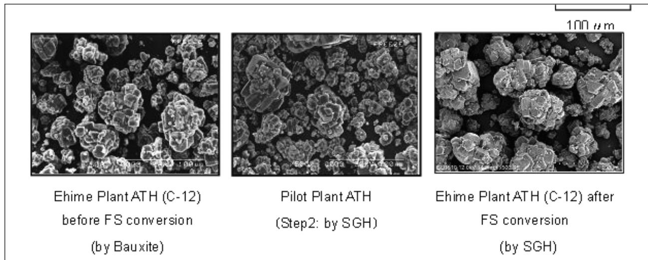
Figure 5. SEM images of Ehime plant ATH (before and after FS conversion) and pilot plant ATH
