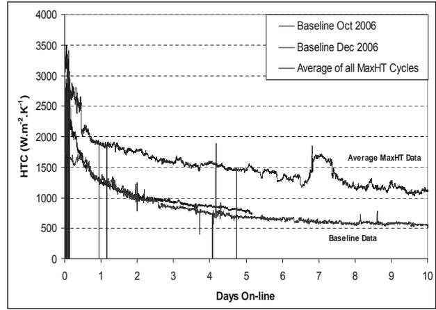
Figure 3: Resistance to Heat Transfer as a Function of Time
