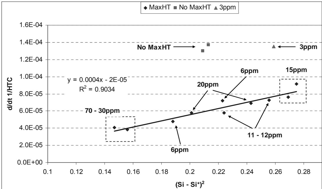
Figure 4: Scaling Rate as a Function of the Square of Silica Supersaturation
