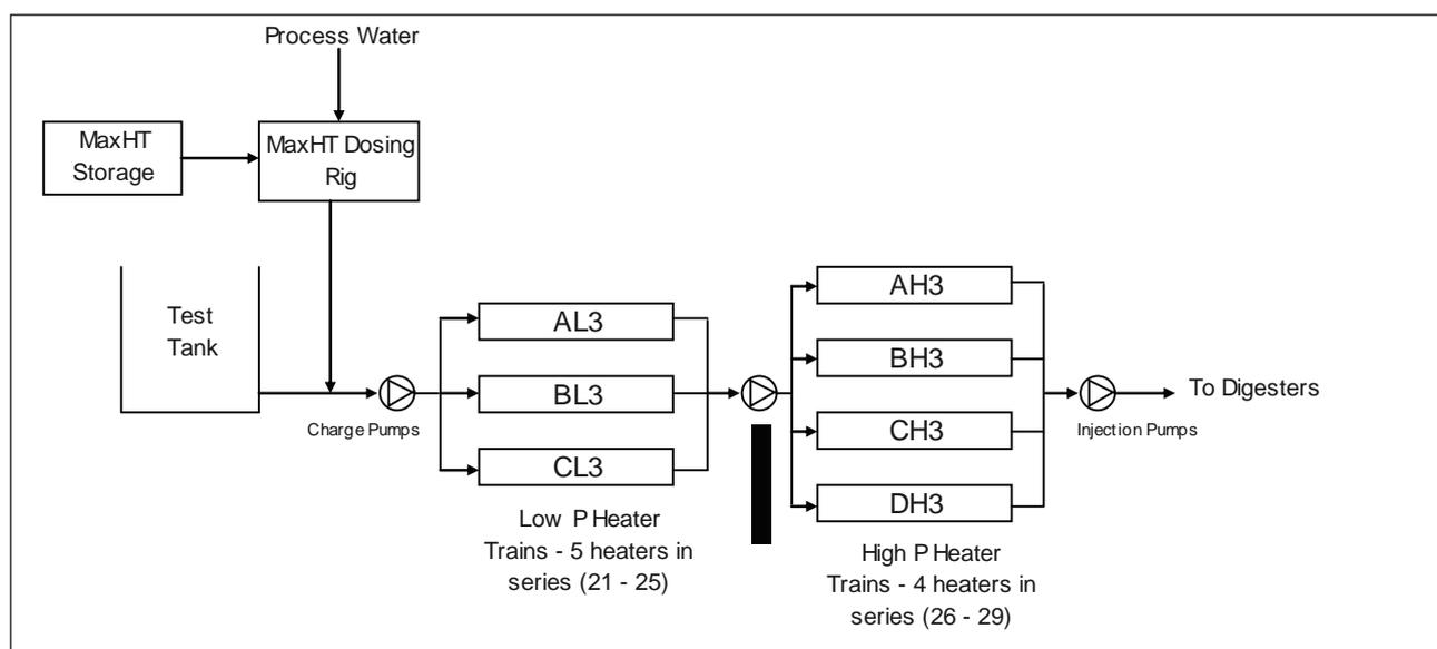
Figure 1: Simplified PFD for Addition of MAX HT® to Unit 3
