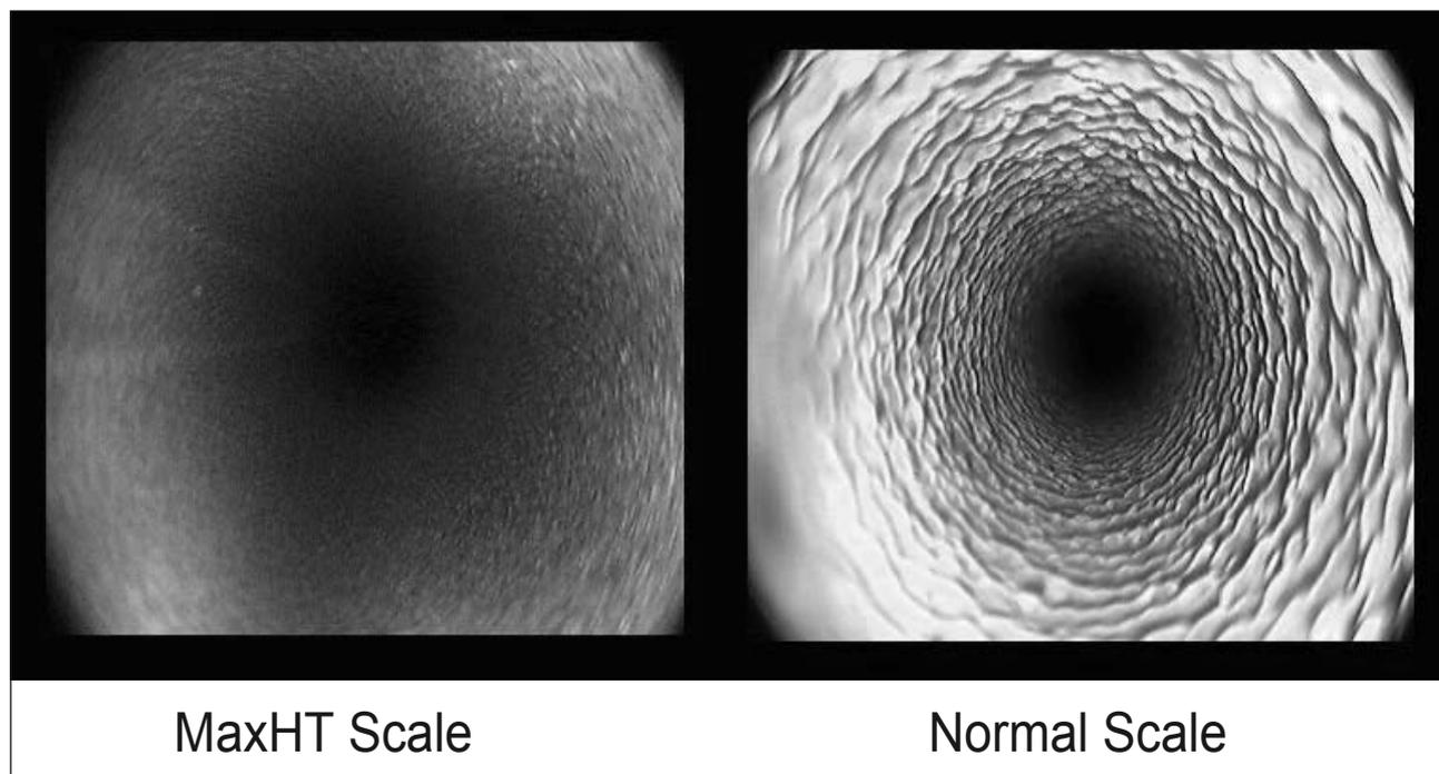
Figure 5: Photos of MAX HT® and Normal Scale within Heater Tubes
