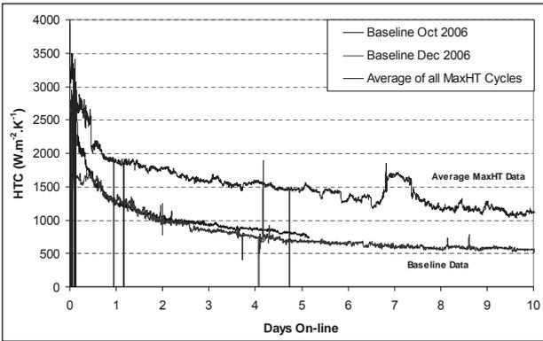
Figure 2: Heat Transfer Coefficient as a Function of Time
