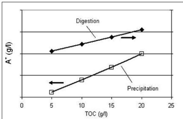
Figure 8. Solubility of gibbsite  $A^*$  at digestion and precipitation conditions in dependence of liquor organics content.
