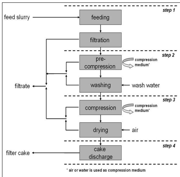
Figure 4. Operation steps of filter press.
