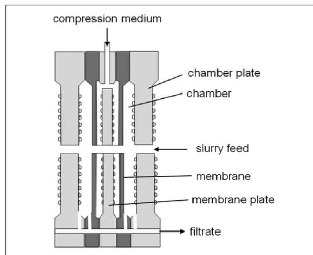
Figure 3. Membrane of filter press.
