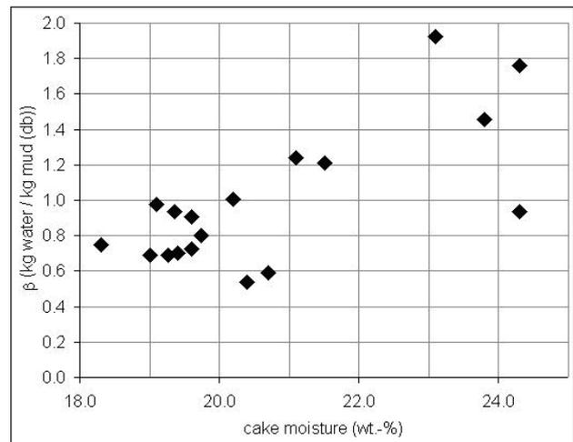
Figure 5. Achieved cake moistures and wash efficiencies during pilot-scale filter tests.
