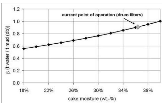
Figure 7. Maximum tolerable specific water consumption in dependence of residue moisture under conditions of constant filtrate flow from filters to last the last washer.
