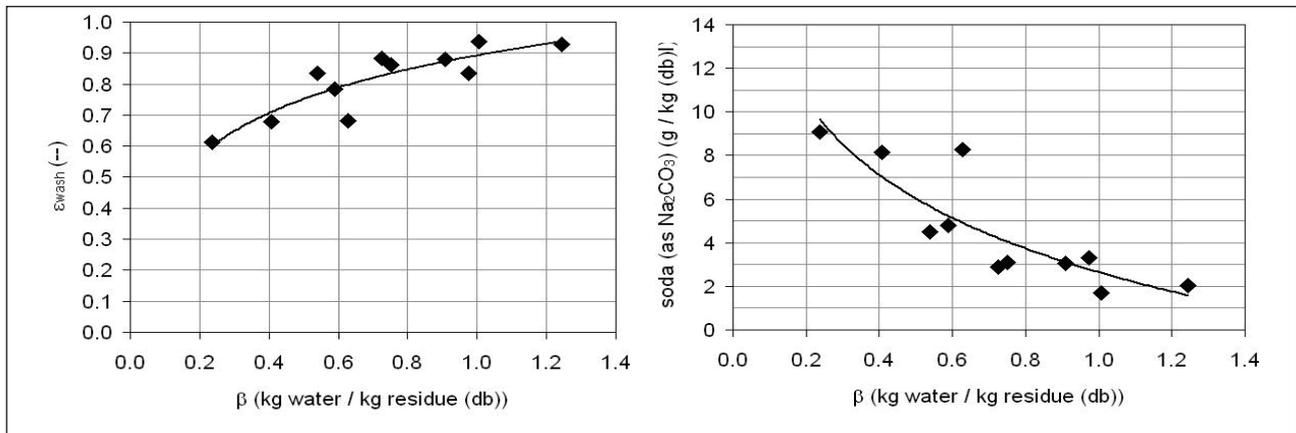
Figure 6. Washing efficiency of the filter (a) and corresponding bauxite residue soda content (b) in dependence of specific water consumption.
