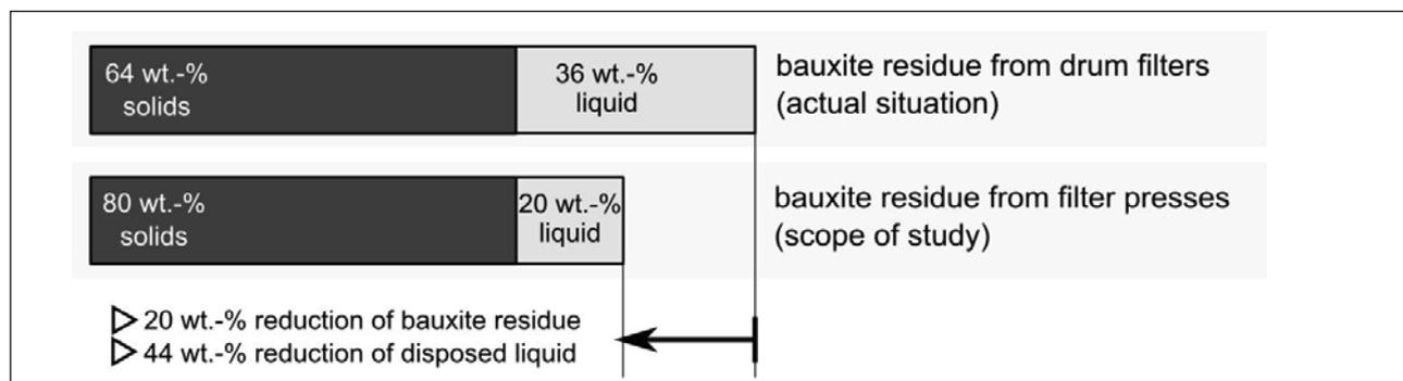
Figure 1. Comparison of bauxite residue from drum filters and filter presses.
