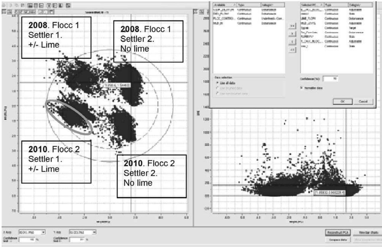
Fig 8. A more complex PCA model illustrating different operating modes for two Settlers
