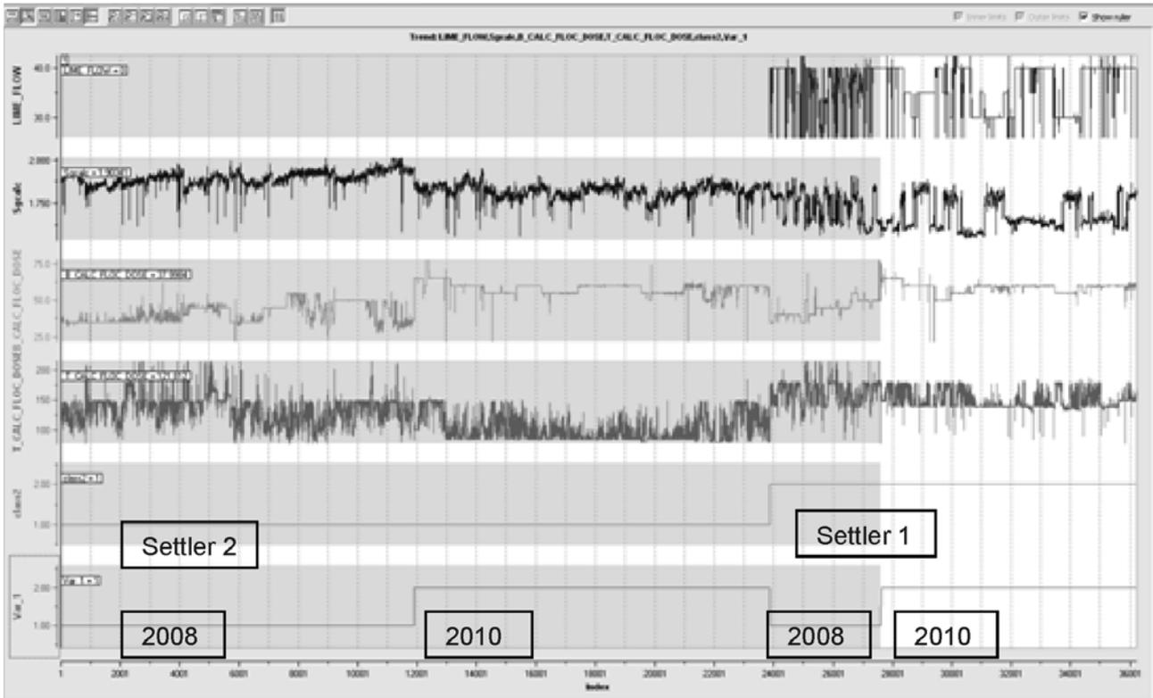
Fig 7. Multiple trends of Lime Rate, U/F Density, Flocculents Addition Rates, Settler Number, and Year
