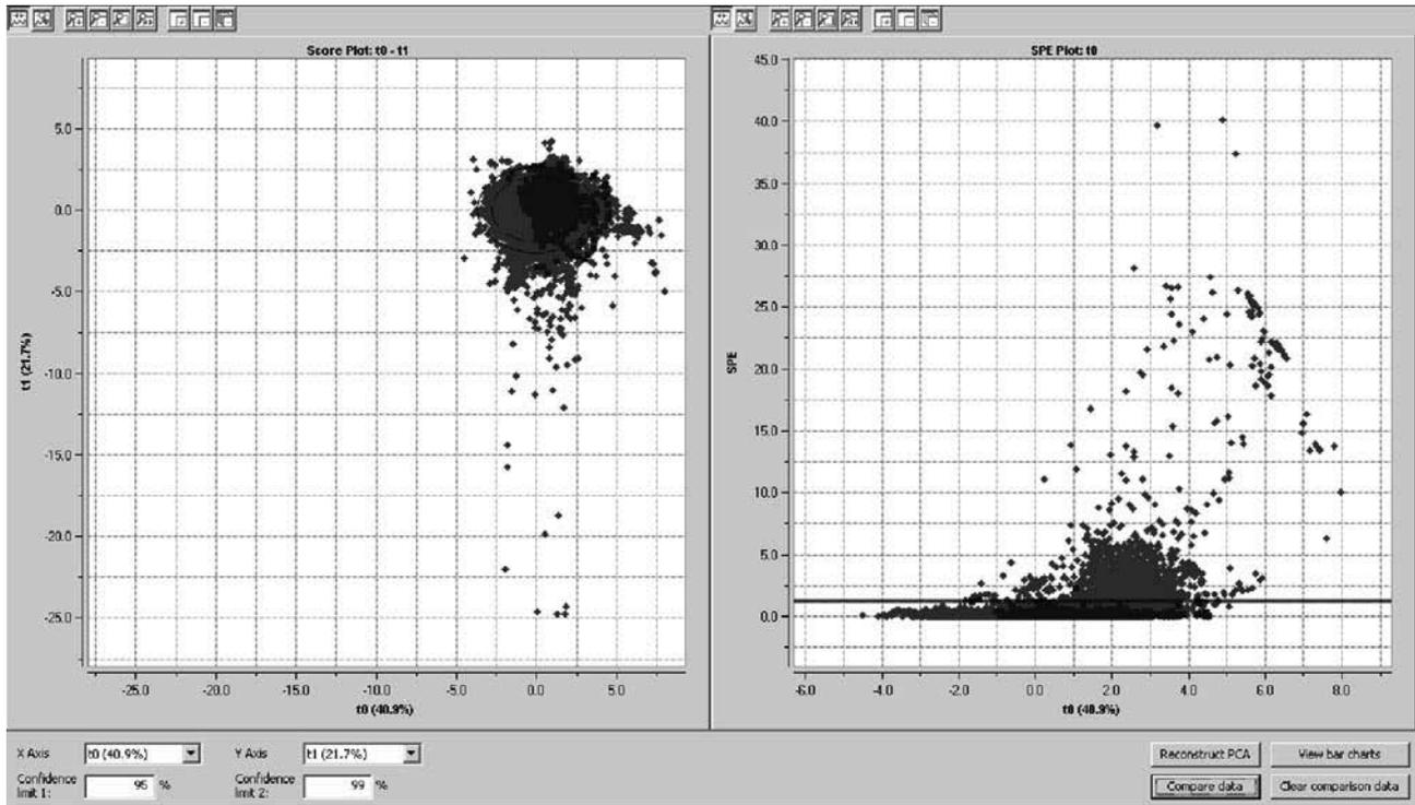
Fig 6. PCA Score Plot and SPE Plot Comparisons for Settler 2. Within the white outline is high rate data
