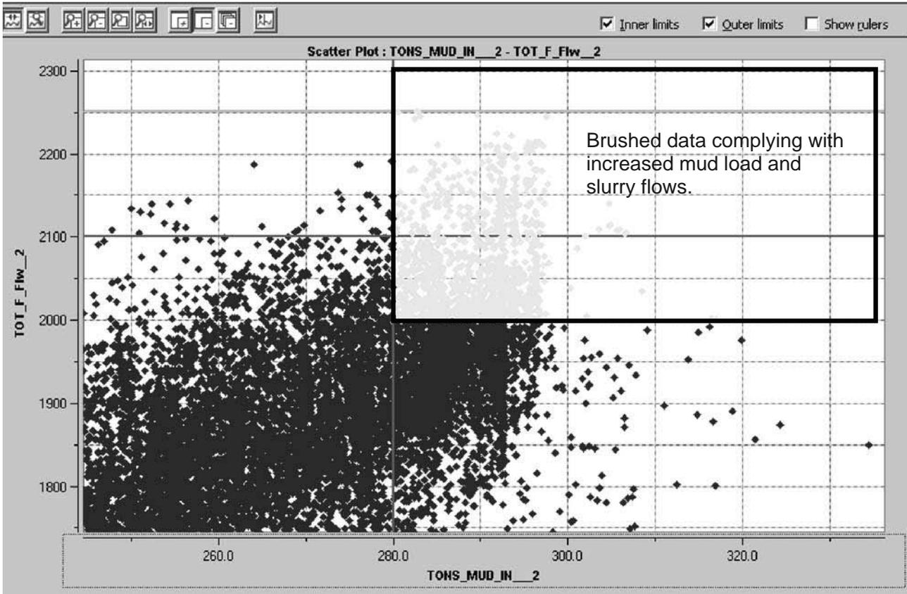
Fig 1. Scatter plot of the two KPI's brushed for the data ranges required.
