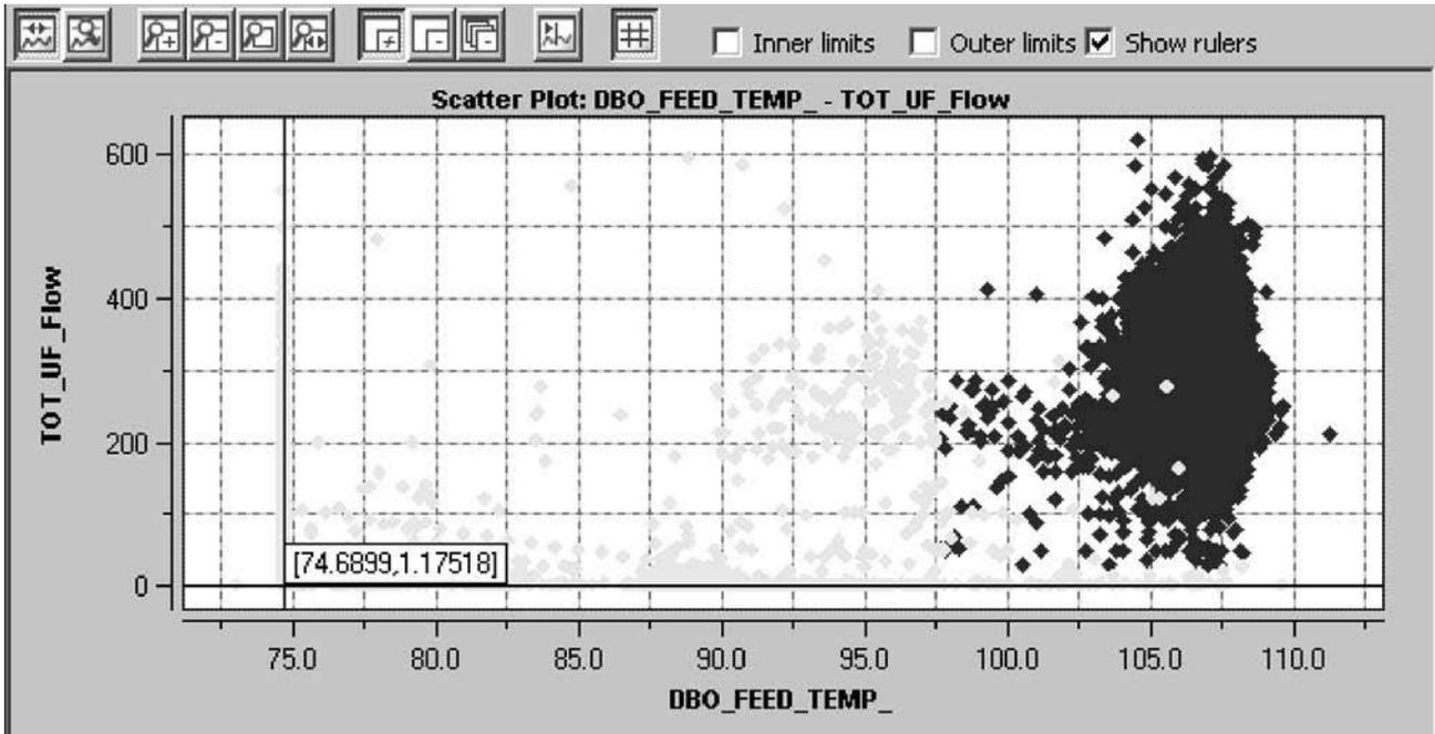
Fig 3. Elimination of low Slurry U/F Rates and low Digestion Temperature data
