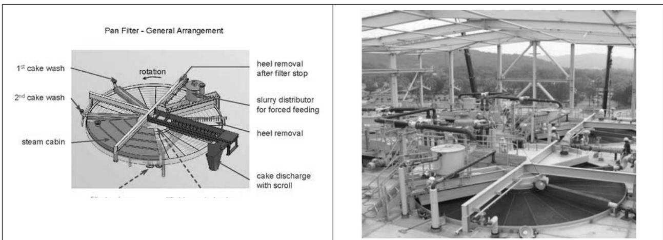
Figure 3: View of a BOKELA product pan filter
