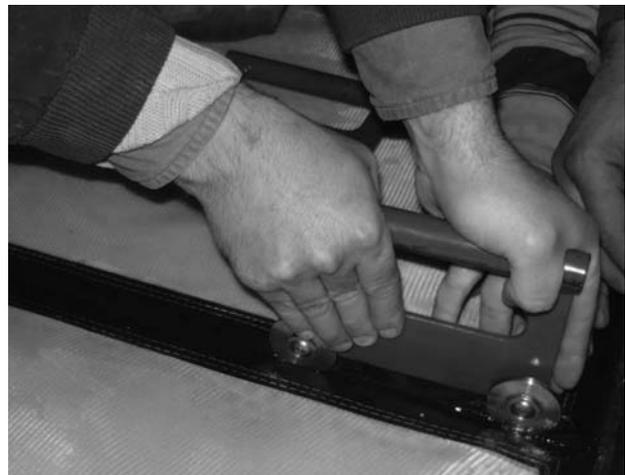
Figure 5: Mounting of FrameTrak™ filter panels on the pan filter - inserting the locking strip with a special tool
