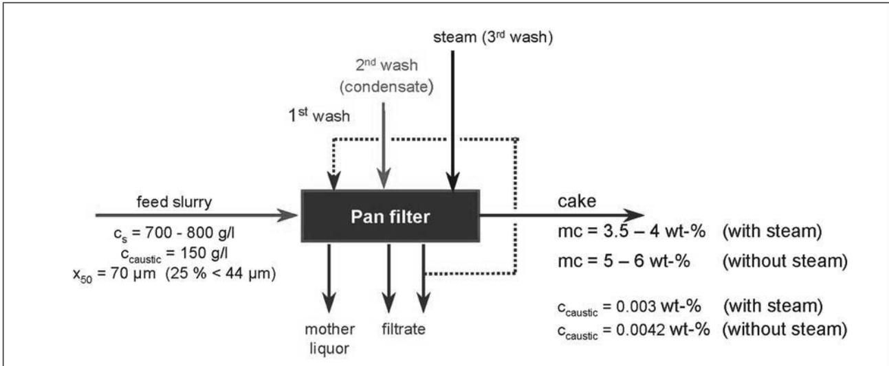
Figure 2: Process scheme and process data of one-step filtration with the new pan filter.
