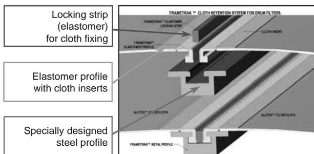
Figure 4: Principle of the cloth retention system FrameTrak™
