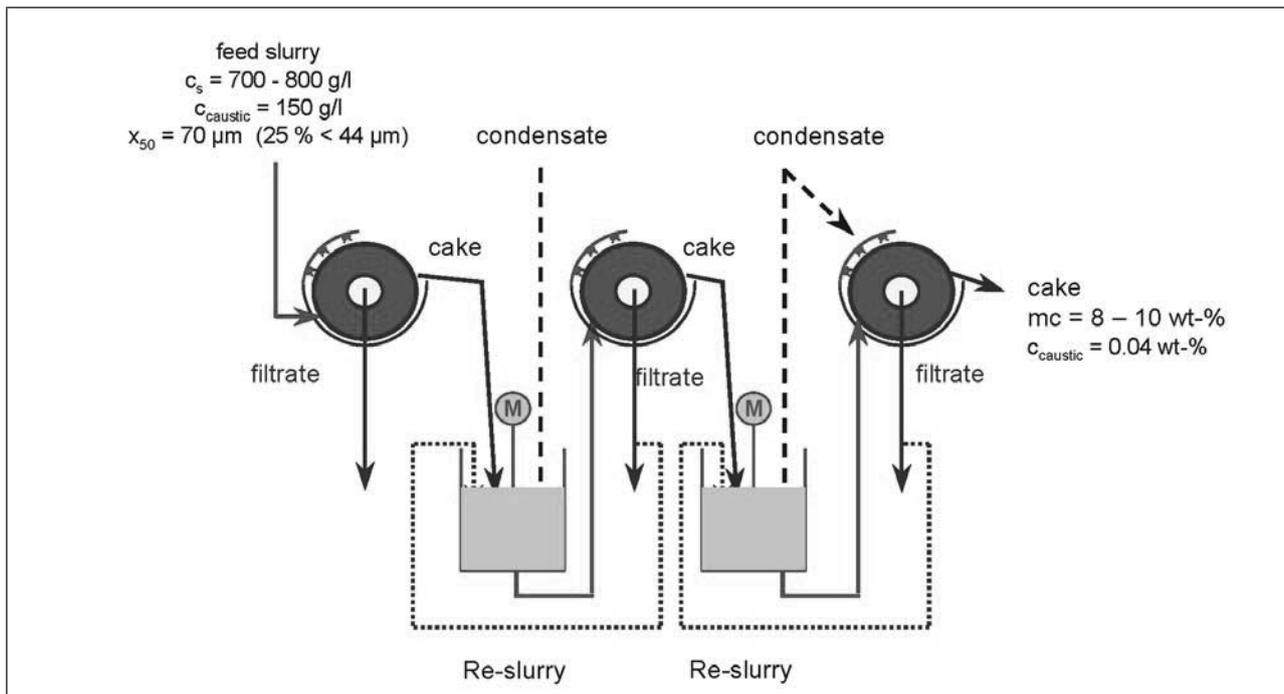
Figure 1: Old plant design and process data of Al-hydrate filtration with three drum filters in series
