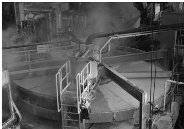
Figure 5: The new pan filter in operation for Al-hydrate product filtration equipped with FrameTrak™
