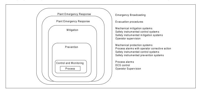
Typical SIS systems in alumina refineries cover overpressure, overtemperature and Burner Management System (BMS) scenarios. The area/unit based SIS systems and associated Safety Instrumented Functions (SIF's) installed during Rio Tinto Alcan's (RTA) refinery upgrade in Gove Northern Territory, Australia is shown below.
