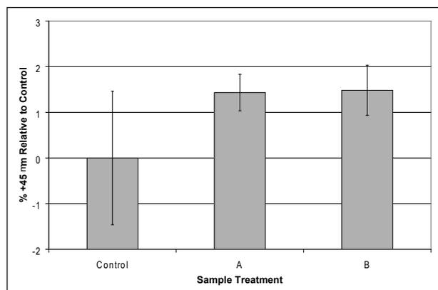
Figure 5. Relative % +45µm sizing data from precipitation bottle tests using seed pre-treated under various conditions as per Figure 3. All treatments had seed exposed to spent liquor for 45 minutes. Control = no CGM addition. Treatment A = CGM added to spent liquor seed slurry. Treatment B = CGM added to spent liquor seed slurry AND to precipitation bottle test liquor. Average of duplicates are shown together with standard deviation.
