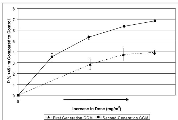
Figure 1. Dose response comparison (relative % +45µm) of a conventional CGM and a new, second-generation product.
