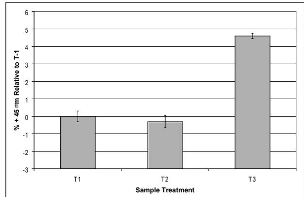
Figure 8. Relative % +45µm sizing data from precipitation bottle tests using LTP liquor exposed to various treatment regimes prior to use in standard precipitation bottle tests. Each liquor was exposed to standard seed for 2 minutes. T1 = no CGM addition. T2 = CGM added to liquor prior to exposure to seed. T3 = CGM added to liquor prior to and after exposure to seed. Average of duplicates are shown together with standard deviation.
