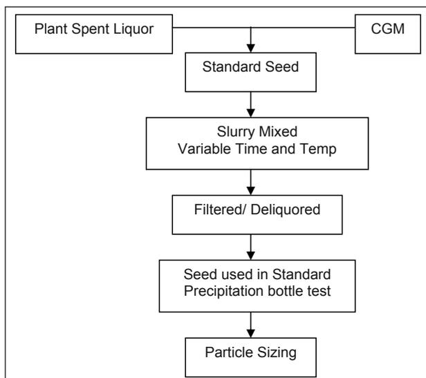
Figure 3. Experimental flow diagram of seed treatment tests.
