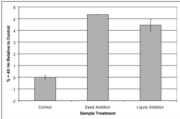
Figure 6. Relative % +45µm sizing data from precipitation bottle tests using seed pre-treated under various conditions. All treatments had seed exposed to spent liquor for 20 minutes. Control = no CGM addition. Seed Addition = CGM added to spent liquor seed slurry. Liquor Addition = CGM added to precipitation bottle test liquor. Average of duplicates are shown together with standard deviation.
