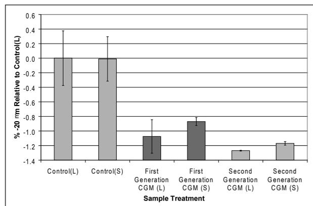
Figure 9. Relative % -20µm sizing data from precipitation bottle tests using seed slurry addition to LTP liquor. Different treatments were defined by addition of CGM to the liquor (L) or the seed slurry (S) prior to mixing of both components. Average of duplicates are shown together with standard deviation.
