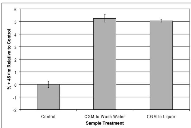
Figure 7. Relative % +45µm sizing data from precipitation bottle tests using seed pre-treated under various conditions. All treatments had seed washed in hot deionised water for 1 minute. Control = no CGM addition. CGM to Wash water = CGM added to water prior to seed addition. CGM to Liquor = CGM added to precipitation bottle test liquor. Average of duplicates are shown together with standard deviation.
