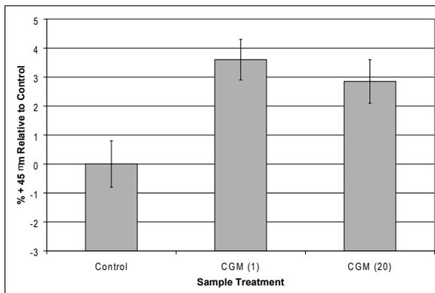
Figure 4. Relative % +45µm sizing data from precipitation bottle tests using seed pre-treated under various conditions as per Figure 3. All treatments had seed exposed to spent liquor for 20 minutes. Control = no CGM addition, CGM (1) had CGM added to spent liquor seed slurry after 19 minutes (1 minute exposure time), CGM (20) had CGM added to spent liquor at the start of the seed treatment (20 minute exposure time). Average of duplicates are shown together with standard deviation.
