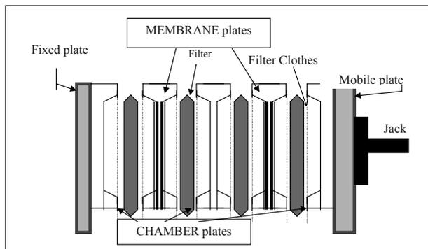
**Figure 2. Configuration of the pilot equipped alternatively with chamber and membrane plates so as to have the cake being squeezed by one side**
