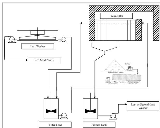
Figure 5. General flow diagram illustrating main flows and operation philosophy of press-filter of Gardanne Alumina Plant
