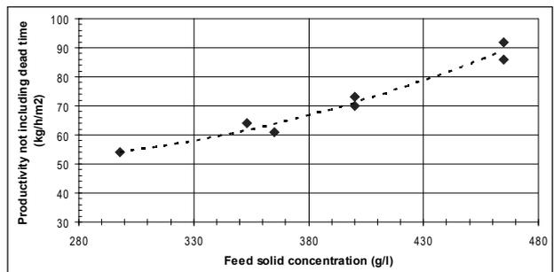
Figure 3. Productivity not including dead time as a function of the feed solid concentration
