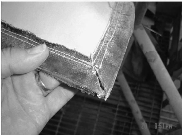
Figure 3. Frame-Trak® gasket splitting at mitred elastomer weld
