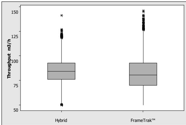
Figure 7. Filter throughput – Box-plot of Frame-Trak® vs hybrid system
