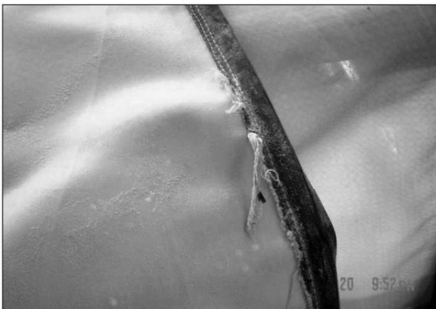
Figure 4. Fraying of Frame-Trak® panel gasket adjacent stitching
