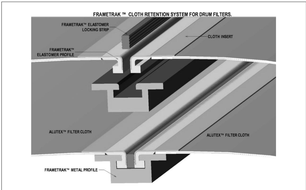
Figure 1. Frame-Trak® Component Assembly
