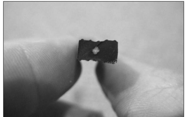
Figure 5. Close-up view of Frame-Trak® locking strip showing rope cord ‘spine’
