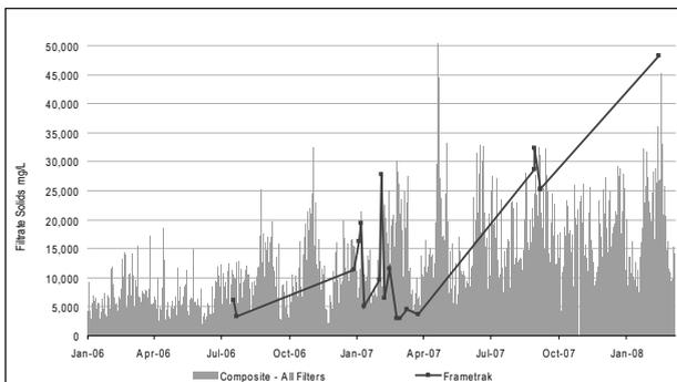
Figure 8. Filtrate solids - Frame-Trak® vs composite sample of all filters
