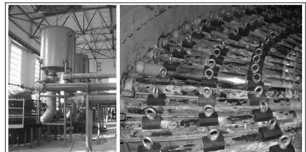
Figure 2. View of BOKELA Backflush Filters with backwash tanks (left), view into the filter with star-shape arranged filter elements (right)
