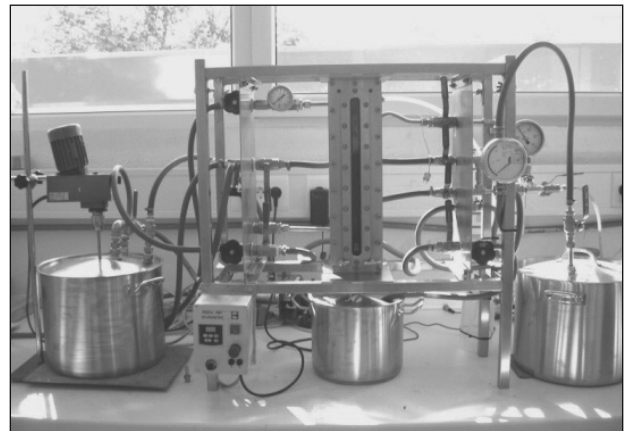
Figure 8. Laboratory test equipment for determination of filtration and backflush characteristics of slurries
