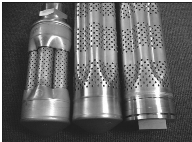
Figure 2. Filter candle design with Bayer liquor candle on the right.
