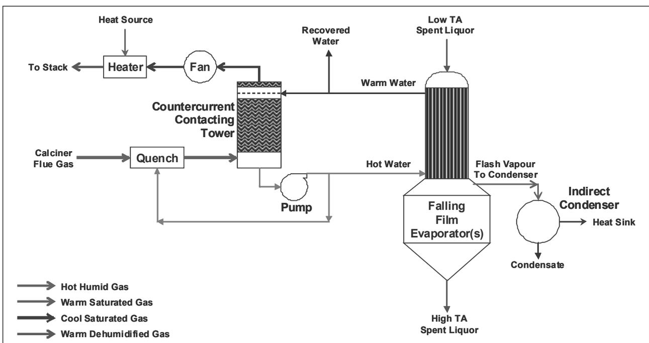
Figure 4. A flowsheet for the recovery of waste heat and water from calciner flue gas.
