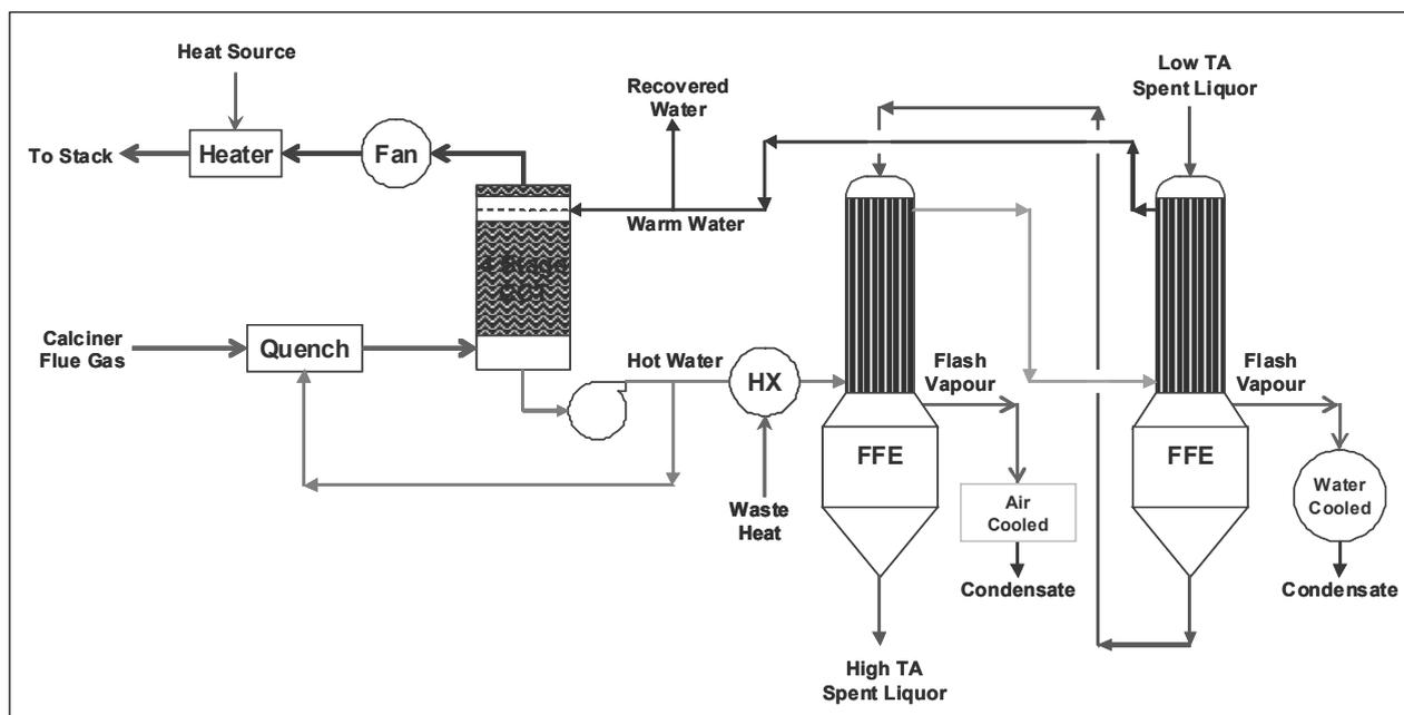
Figure 6. Calciner waste heat recovery with air cooled condensers for greater water recovery.
