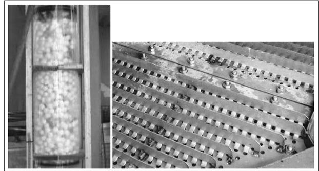
Figure 5. (a) Pilot scale Turboscrubber and (b) impingement tray for tray tower (Lisbon Engineering, with permission).
