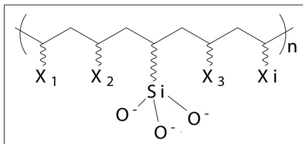
Figure 1. Generic structure for MAX HT Sodalite Scale Inhibitor
