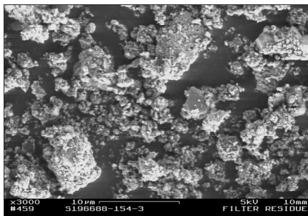
Figure 5. SEM image of test tank liquor solids.
