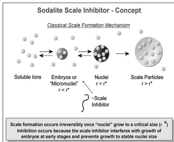
Figure 2. Proposed antiscalant mechanism for MAX HT Sodalite Scale Inhibitor
