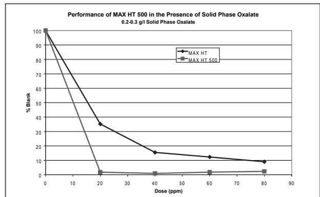
Figure 10. MAX HT performance with solid phase oxalate.
