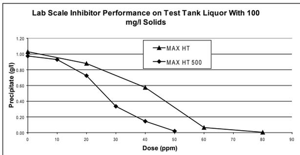
Figure 7. Lab test comparing MAX HT 500 to first generation MAX HT
