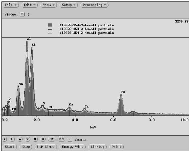
Figure 6. EDX spectrum on smaller particles.
