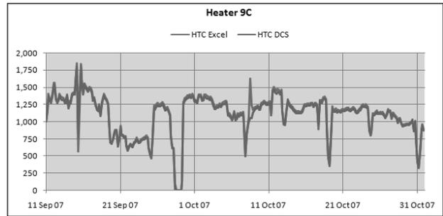
Figure 8. Live steam heater treated with MAX HT 500 (dose 50 ppm at start, reduced in stages to 25 ppm on Day 27).
