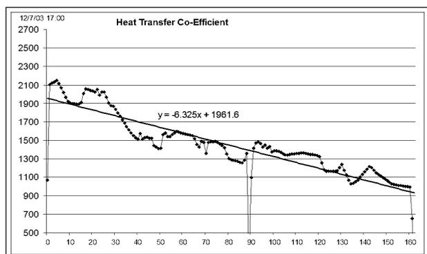
Figure 3. Typical heat transfer decay during ~7 days when no antiscalant was used.
