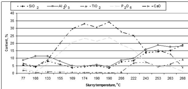
Figure 3. Elemental distributions in the scale samples versus slurry temperature
