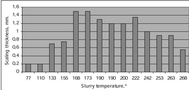
Figure 2. Scaling of the heating surface versus slurry temperature
