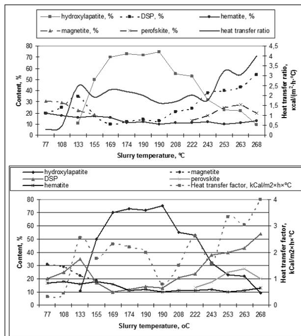
Figure 8. Phase distributions and heat transfer ratio of the deposits versus slurry heating temperature
