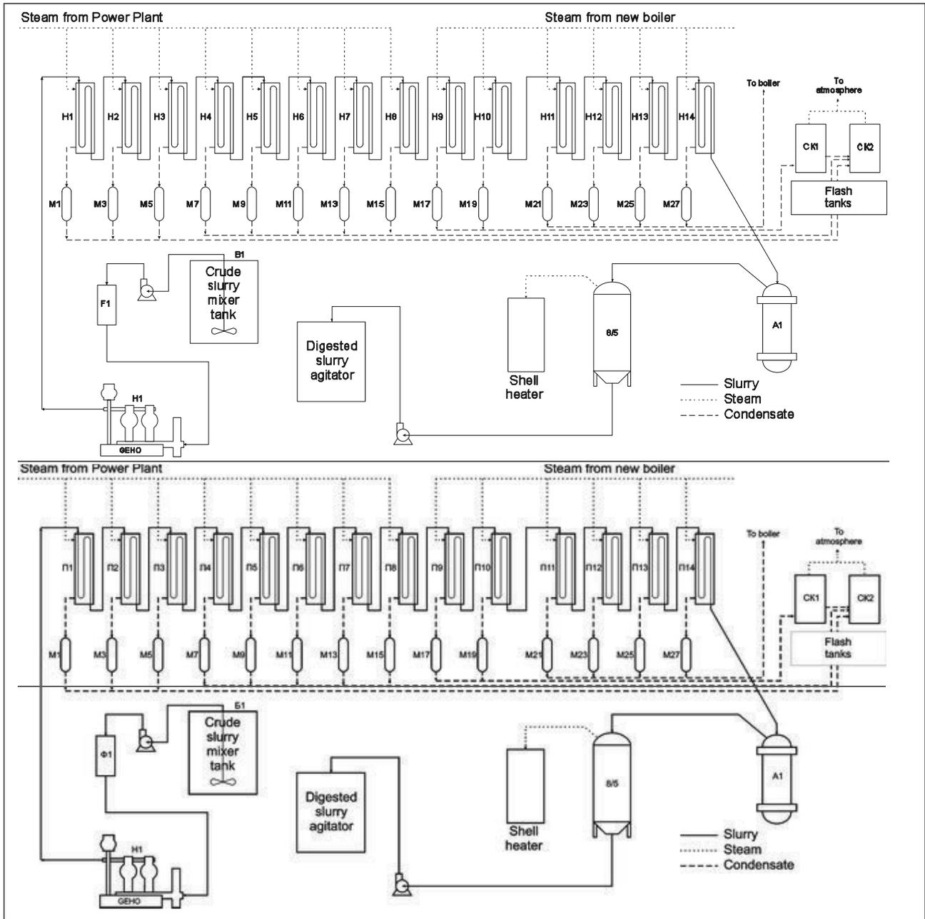
Figure 1. Process block diagram of TU HTD
