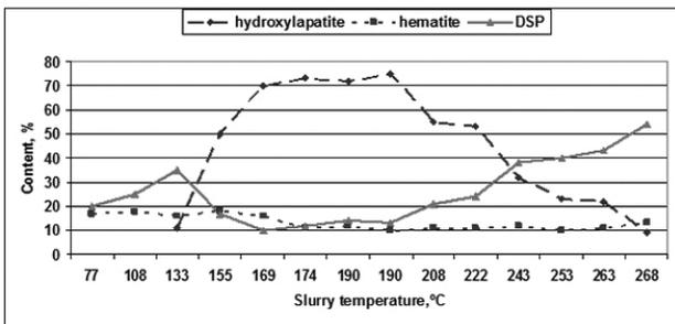
Figure 4. Distribution of hydroxylapatite, hematite and DSP in the scale samples versus slurry temperature
