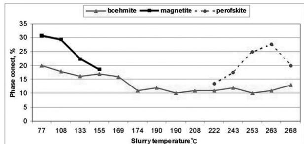
Figure 5. Distribution of magnetite, boehmite and perovskite in the scale samples versus slurry temperature
