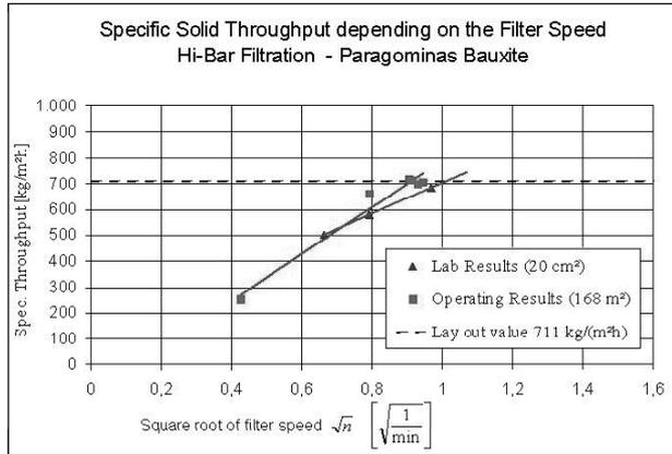
Figure 5. Specific solids throughput of the hyperbaric filters in operation compared to scale-up throughput value calculated by BOKELA (same granulometry of real slurry and test material)
