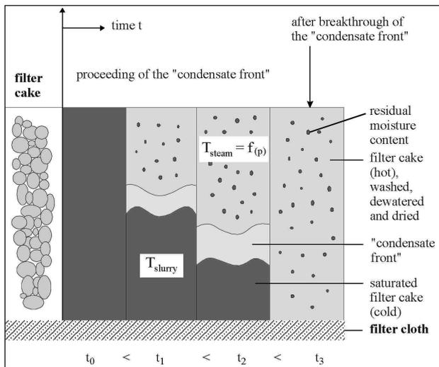
Figure 3. Steam Pressure Filtration: model of the “condensate front”
