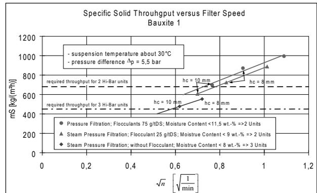
Figure 7. Specific solids throughput as function of square root of the filter speed (filter layout for moisture content  $mc < 11.5 \text{ wt\%}$ )
