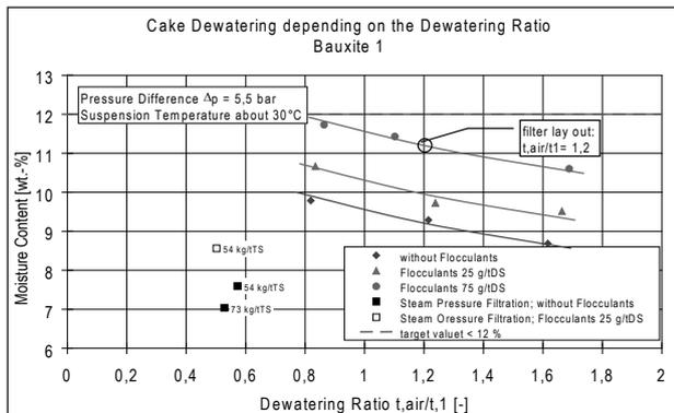
Figure 6. Moisture content as function of the dewatering ratio  $t_2/t_1$  ( $t_2$  = dewatering time,  $t_1$  = cake formation time) for a pressure difference  $\Delta p = 5.5 \text{ bar}$
