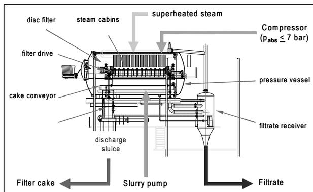
Figure 1. Schematic view of a Continuous Pressure Disc Filter with steam cabins for steam pressure filtration
