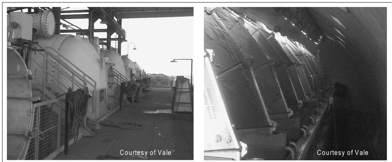
Figure 4. View of the filter plant with five continuous pressure disc filters ( $168\text{m}^2$  filter area each, 12 discs and 240 sectors i.e.20 sectors per disc) (left); view into a pressure vessel (right)
