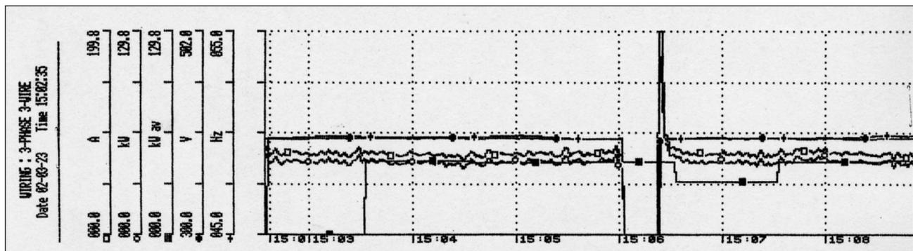
Figure 9. Restart of the agitator after 20 s
