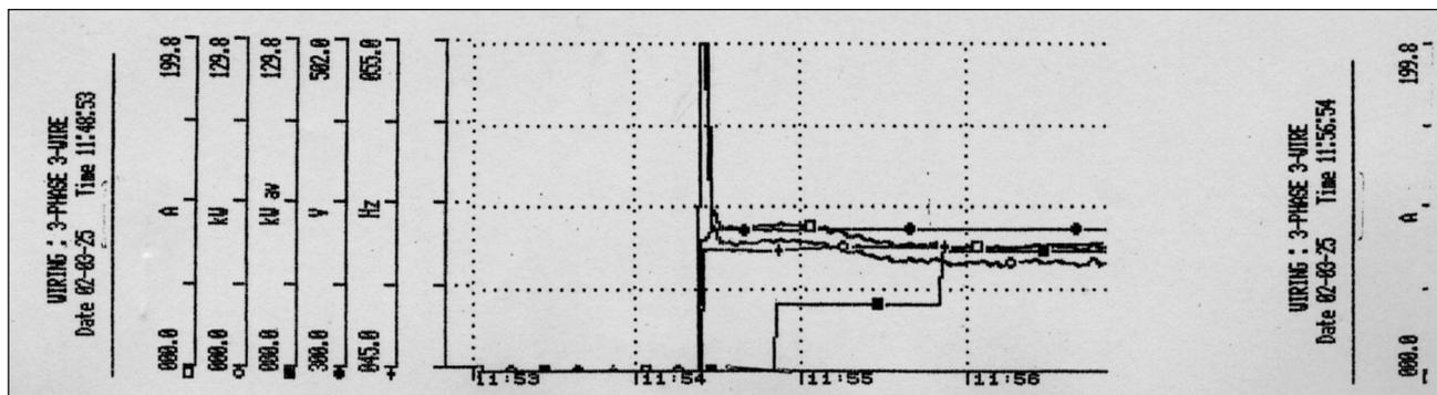
Figure 10. Restart of the agitator after 30 minutes
