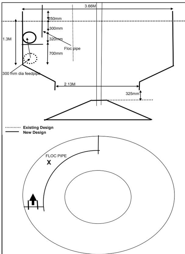
Figure 4. Showing the initial changes that were made to improve the performance of the tank.
