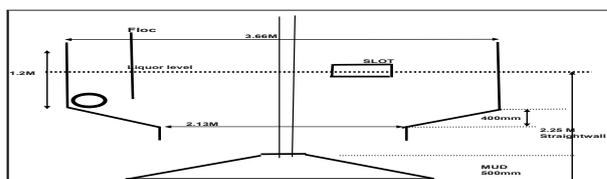
Figure 3. Basic design of feedwell installed in 30.5 meter diameter Kirkvine tanks 2005-2006.
