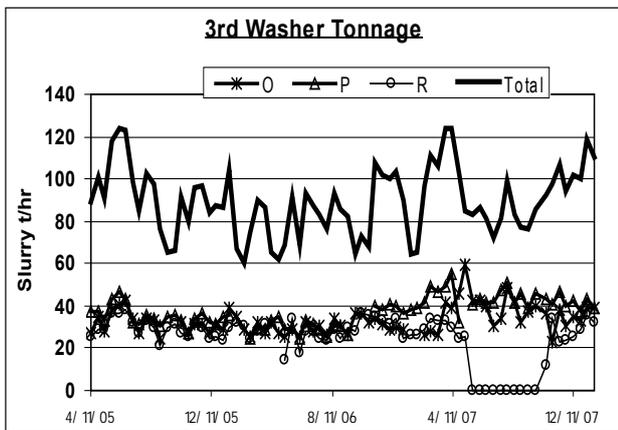
Figure 5. Plot of third washer underflow tank tonnages.
