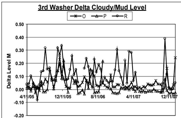
Figure 7. Third washer delta cloudy/ mud level showing the improved performance of O and P after being modified.
