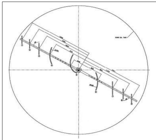
Figure 11. Plan view of reduced rake blade design.
