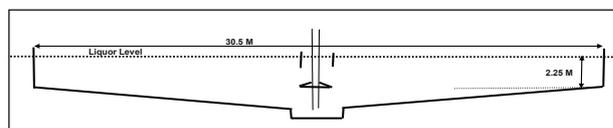
Figure 2. Basic design of 1<sup>st</sup> and 3<sup>rd</sup>stage washers
