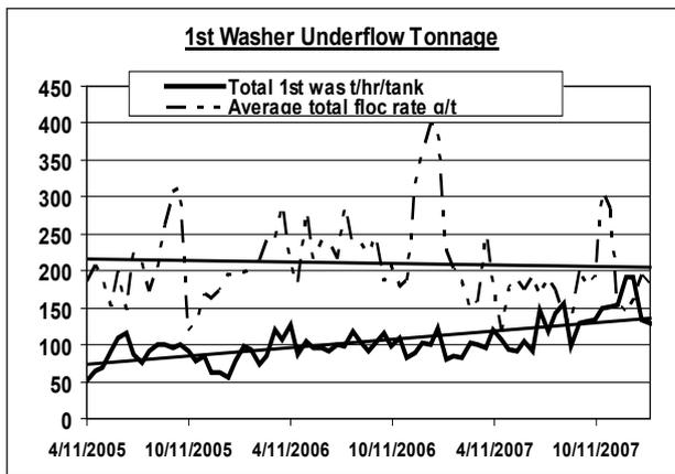
Figure 9. Decreasing flocculant usage and increasing tonnage.
