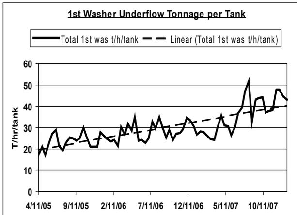
Figure 8 Increasing average tonnage handled by each first washer.
