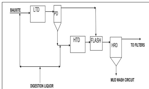
Figure 3. Cross-Flow Double Digestion Flowsheet
