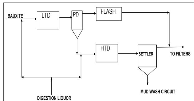
Figure 2. Parallel Double Digestion Flowsheet
