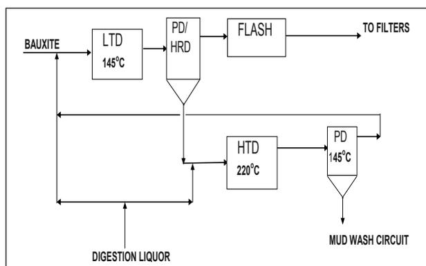
Figure 4. Counter-current Double Digestion Flowsheet
