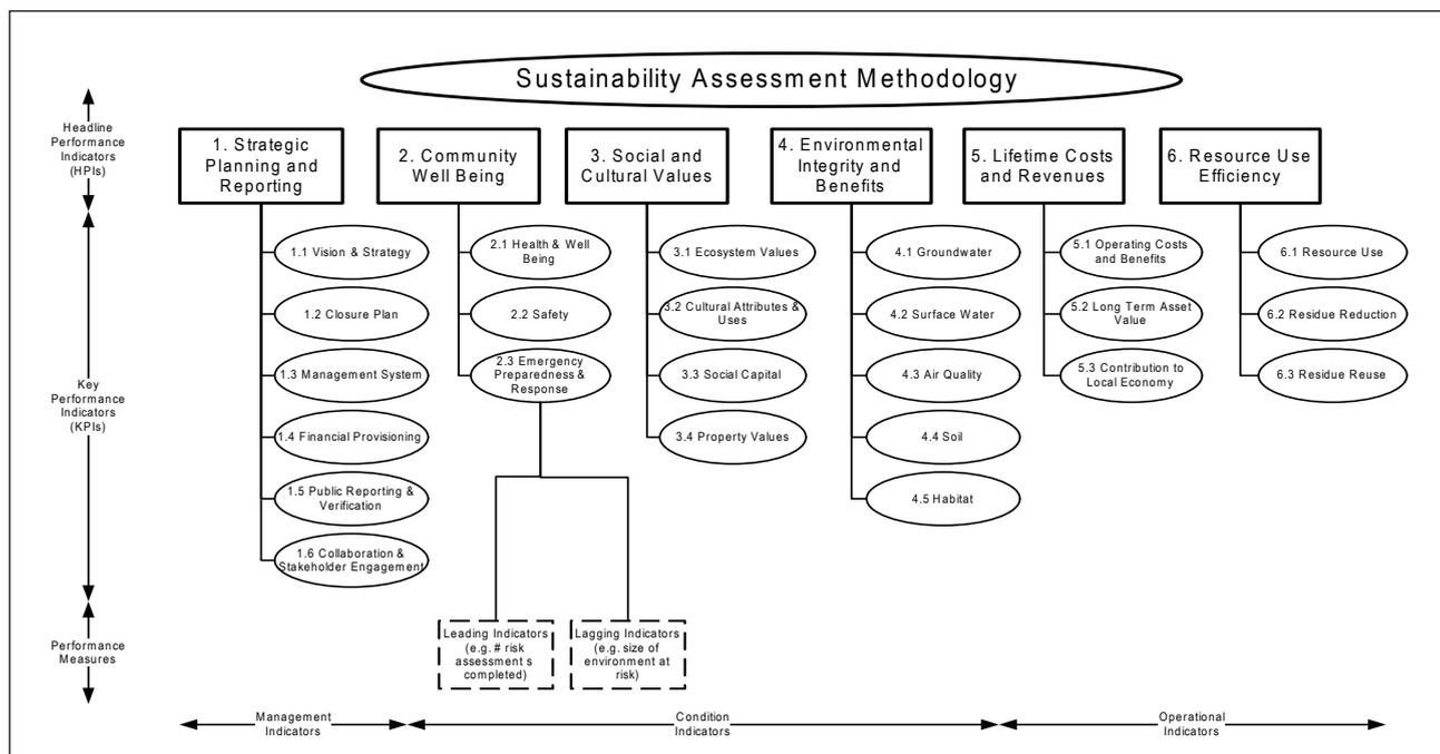
Figure 2. Overview of the indicator system for the sustainability assessment of bauxite residue management (Source: (Van Berkel et al. 2007)).
