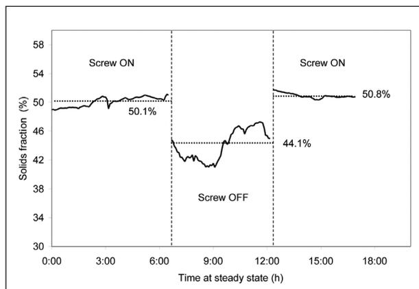
Figure 3. Underflow solids with the screw on and off
