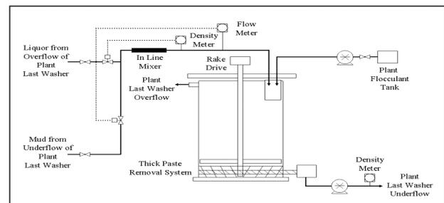
Figure 1. Diagram of the screw thickener with the thick paste removal system and auxiliary equipment
