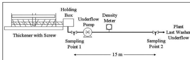
Figure 5. Sampling points at the underflow of the pilot thickener
