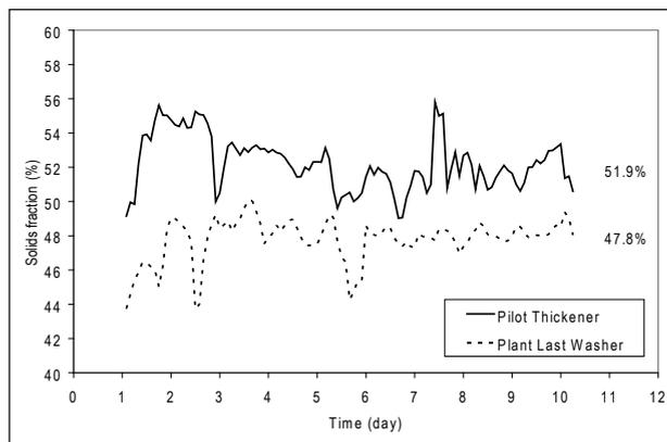
**Figure 6. Comparison of underflow solids for the pilot thickener and for the plant last washer**
