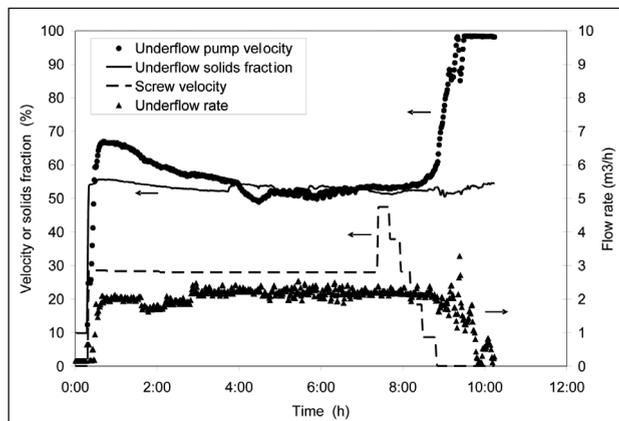
Figure 2. Impact of the screw velocity on the underflow of the thickener
