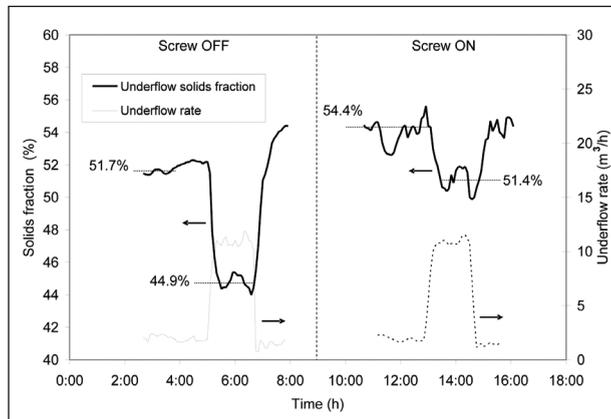
Figure 4. Impact of the underflow rate on underflow solids fraction with the screw off and on
