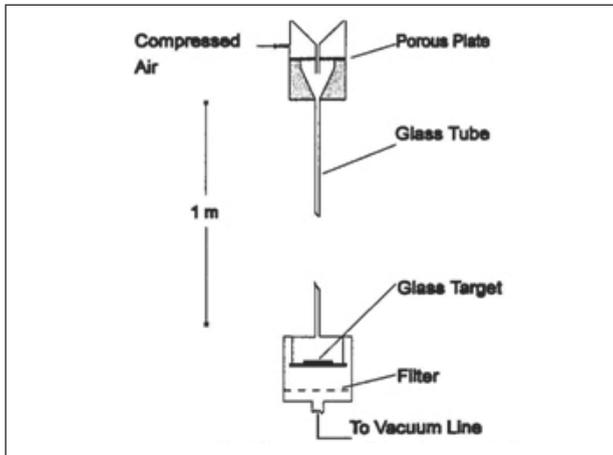
Figure 1. Ghadiri test apparatus (from [3]).
