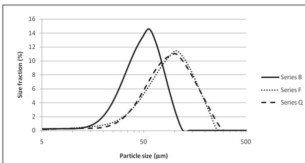
Figure 2. Initial size distribution of alumina test samples.
