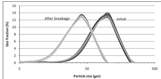
Figure 3. Repeatability of test results for Series Q (13 samples of as-received (initial) and 15 samples attrited under nominally identical conditions)
