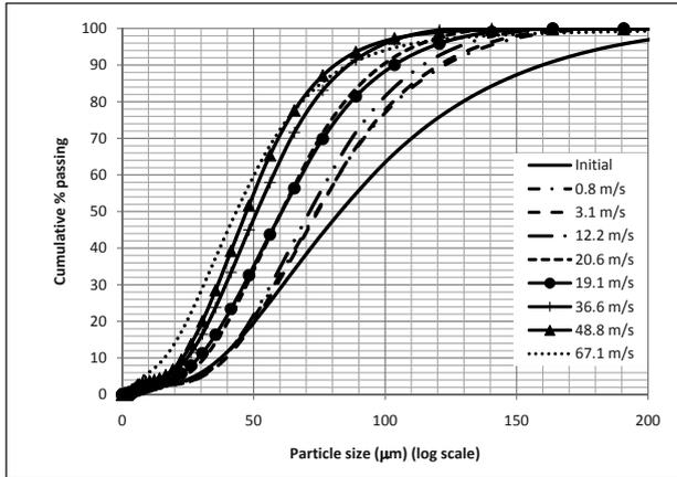
Figure 7. Effect of air stream velocity on particle breakage for Series Q.
