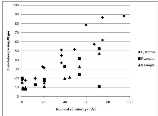
Figure 8. Effect of air stream velocity on fraction of particles passing 48 µm.
