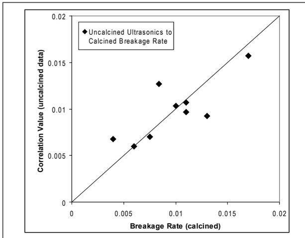
Figure 6a. Uncalined longitudinal velocity and bulk density measurements correlated to calcined breakage rate.
