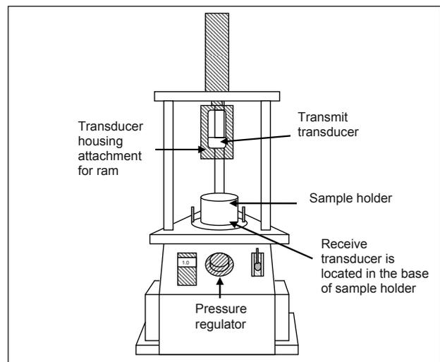
Figure 2. Schematic of measurement apparatus. Note: longitudinal transducer pair is shown in this figure. Schematic of shear transducer pair for use in the same apparatus (with transducer housing attachment for ram removed) is shown in Figure 3B.
