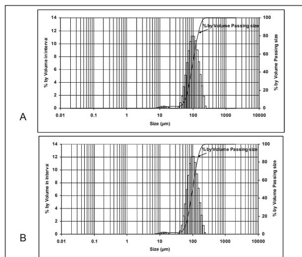
Figure 4: Size distribution of alumina (a) before measurement procedure and (b) after measurement procedure. Note: Size cut-point results from the graphs are summarised in Table 2.
