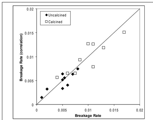
**Figure 5a. Comparison of predicted to actual breakage rate for calcined and uncalcined alumina using longitudinal ultrasonic measurements.**
