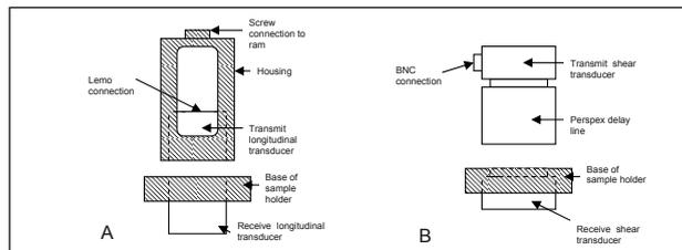
Figure 3. Schematic of transmit and receive transducer pairs for (A) longitudinal measurement, and (B) shear measurement.
