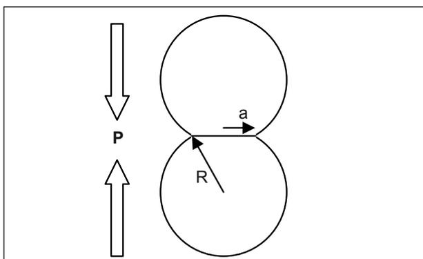
Figure 1. Two spheres of radius  $R$  in contact under pressure  $P$  have a contact area of radius  $a$ .
