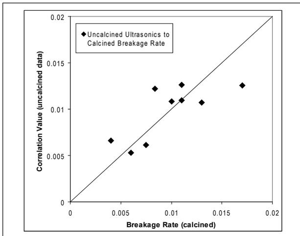
Figure 6b. Uncalined shear velocity and bulk density measurements correlated to calcined breakage rate.
