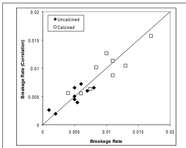
**Figure 5b. Comparison of predicted to actual breakage rate for calcined and uncalcined alumina using shear ultrasonic measurements.**
