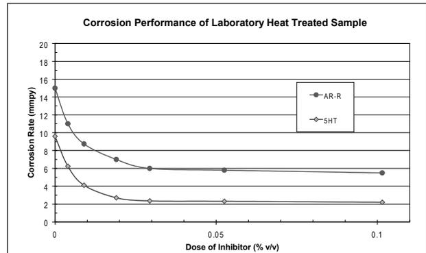
Figure 7. Corrosion Performance of sample 5HT
