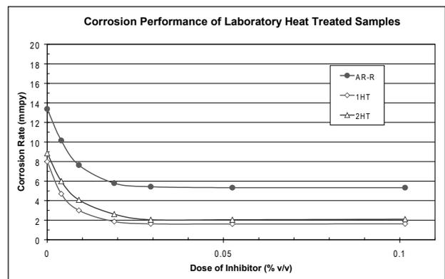
Figure 1. Corrosion Performance of sample 1HT & 2HT
