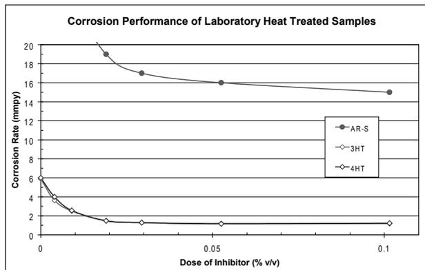
Figure 4. Corrosion Performance of sample 3HT & 4HT
