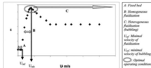
Figure 3. Evolution of the alumina fluidized bed void fraction ( $\epsilon$ ) with the fluidization velocity ( $U$ )
