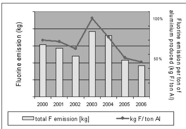
Figure 5. Contribution of HDPS dosing technology to Fluorine (F) emission reduction: GTC industrial results on AP potline technology
