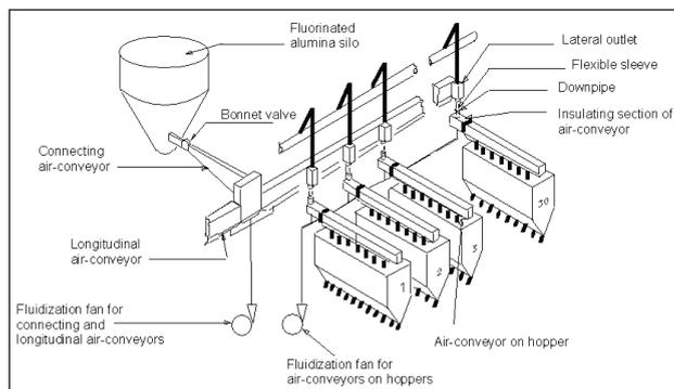
Figure 1. General HDPS pot feeding arrangement
