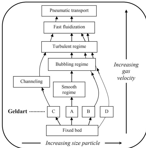
Figure 4. Progressive change in gas contacting with change in gas velocity
