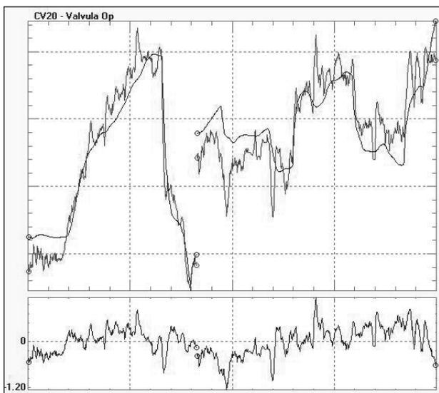
Figure 7. Valve Opening Prediction.
