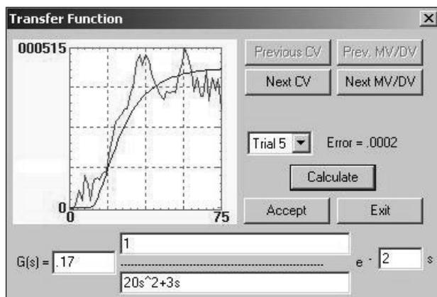
**Figure 2. Model of one of the mass balance variables (MV) and the alumina-caustic concentration Ratio (CV).**
