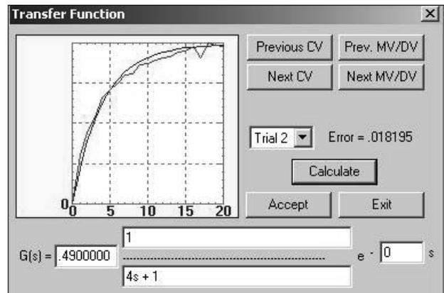
**Figure 3. Valve modeling against the steam flow.**
