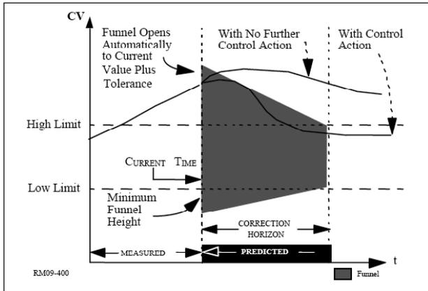
Figure 1. RCA technique controlling a CV inside limits.
