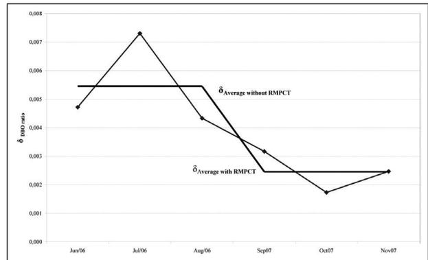
Figure 8. Behaviour of DBO ratio standard deviation ( $\delta_{DBO}$ ) with and without RMPCT operation.
