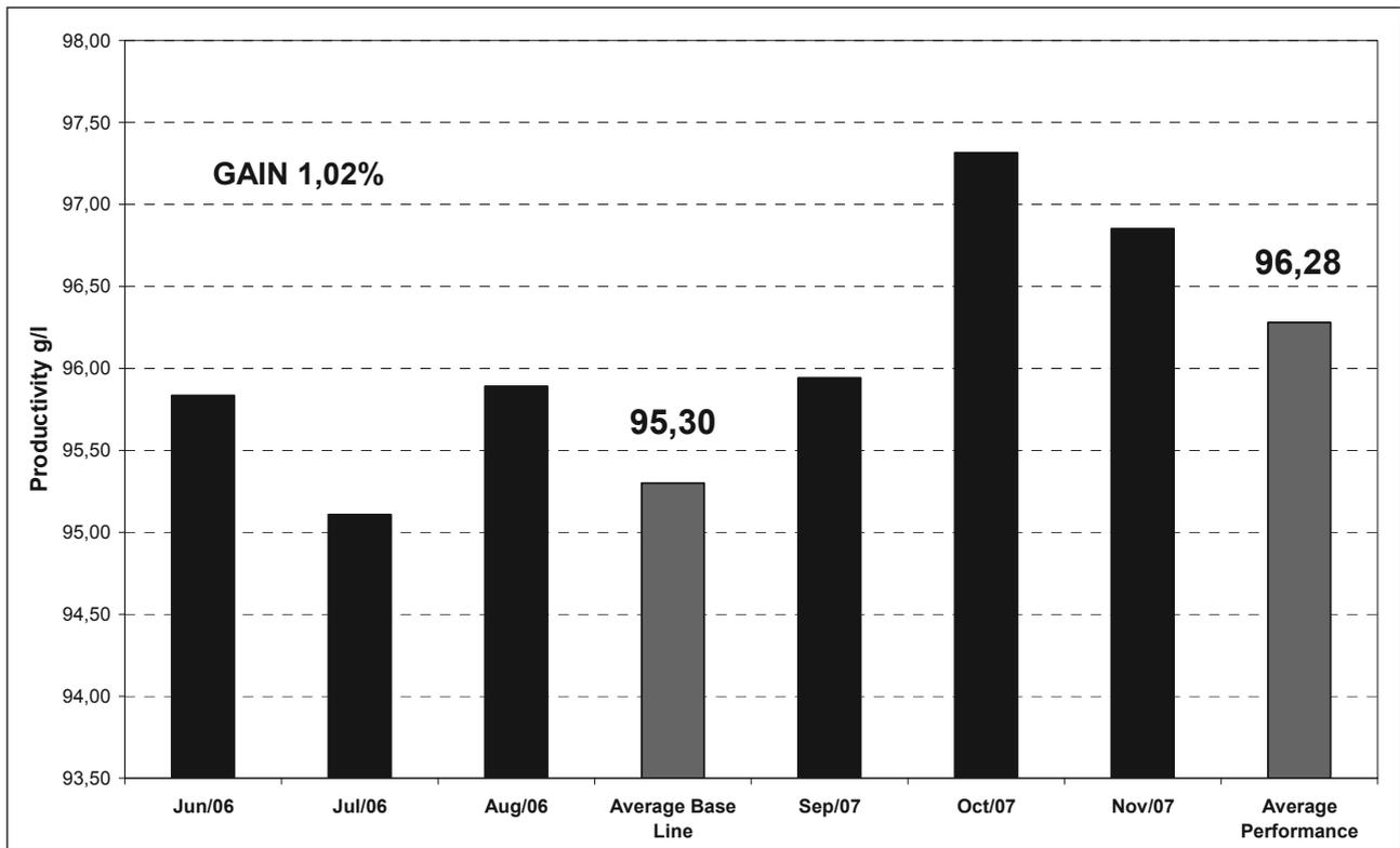
Figure 9. Behaviour of productivity in digestion system with and without RMPCT operation.
