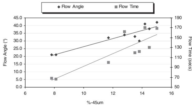
Figure 2 – Flow Properties of Secondary Alumina
