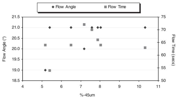
Figure 3 – Flow Properties of Primary Alumina
