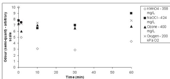
Figure 2. Kinetic test results (Worsley Alumina condensate). T= 90°C, pH = 10.6, stirring speed = 800 rpm. Note – ozone concentration based on quantity of ozone passed through condensate – amount of ozone dissolved in solution was considerably lower.
