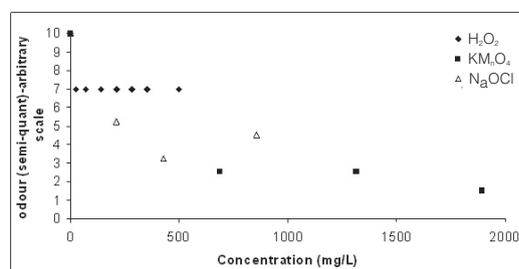
Figure 1a. Effect of oxidant concentration on odour removal.  $T = 90^\circ C$ ,  $pH = 10.6$ ,  $t = 1h$ , tests conducted in culture tubes rotating in water bath.
