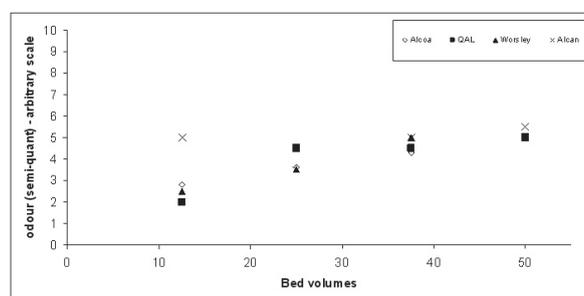
Figure 4. Removal of odour from different alumina refinery condensates using powdered activated carbon adsorption. T=90°C, residence times = 9.6 – 12.6 sec, pH = 10.6 ± 0.2.
