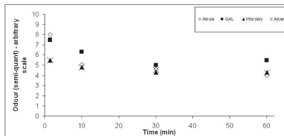
Figure 3. Removal of odour from different alumina refinery condensates using KMnO<sub>4</sub> oxidation. T= 90°C, pH = 10.6 ± 0.2, stirring speed = 800 rpm, [KMnO<sub>4</sub>] = 358 mg/L
