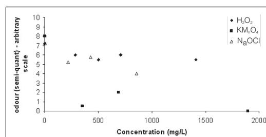
Figure 1b. Effect of oxidant concentration on odour removal.  $T = 90^\circ C$ ,  $pH = 5$ ,  $t = 1h$ , tests conducted in culture tubes rotating in water bath.
