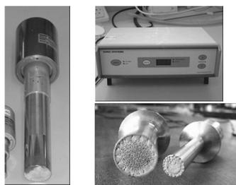
Figure 3: Laboratory based ultrasonic equipment (Left: 20kHz probe, Top right: ultrasonic generator, Bottom right: the damage to probes following 30h non-continuous ultrasound applied when immersed in water at 20°C)
