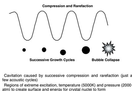
Figure 1: The effects of acoustic cavitation upon a liquid medium
