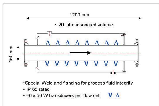
Figure 6: C<sup>3</sup> 1 m section shown with bonded transducers
