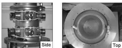
Figure 2: C<sup>3</sup> Proprietary Ultrasonic Flow Cell (Perkins 2000)
