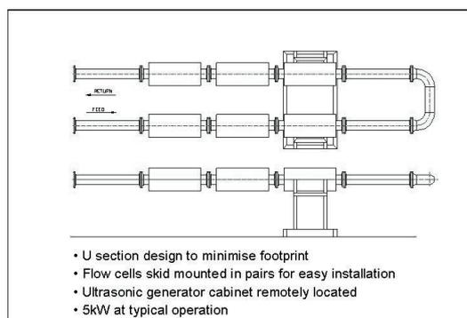
Figure 7 : Left: Schematic of full scale system; Right (7B): Actual plant installed equipment
