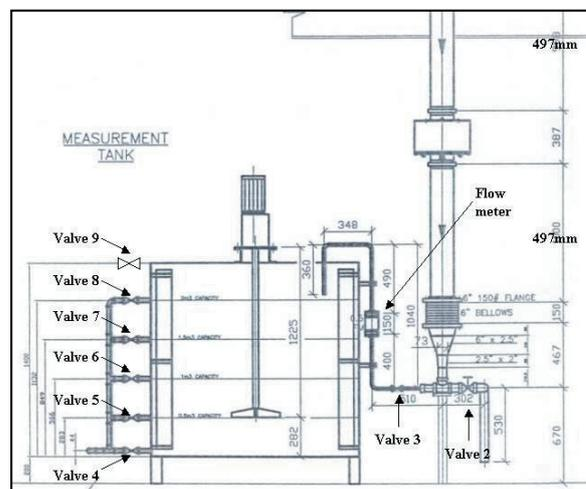
Figure 4: Process drawing for the C<sup>3</sup> Flow-cell linked to the temperature controlled 2m<sup>3</sup> stirred tank
