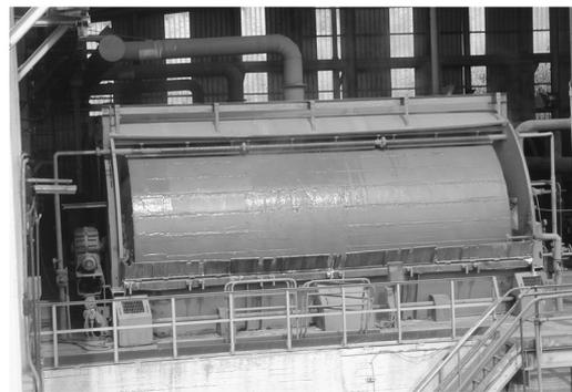
Figure 5: Cake washing before modification (the wash water is not equally distributed and runs down the drum to the cake discharge zone)
