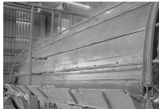
Figure 6: Cake washing on the modified filter with new washing system provides for good wash liquor distribution
