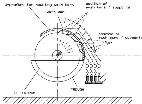
Figure 4: New arrangement of wash bars
