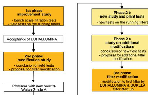
Figure 1: Schedule of the red mud drum filter optimisation by BOKELA and EURALLUMINA at the Portoscuso Alumina refinery
