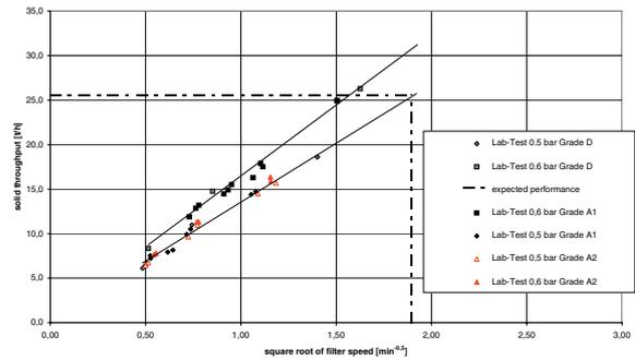
Figure 2: Theoretical throughput rate of three types of bauxite (bauxite A1 = 70 % grade A and 30 % grade D, A2 = 100 % grade A, D = 100 % grade D)
